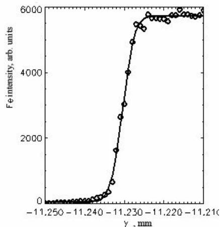
Fig. 3. Fit of error function to horizontal scan over lithographic structure.
