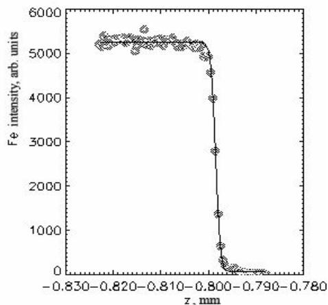
Fig.2 Fit of error function to vertical scan over lithographic structure.
