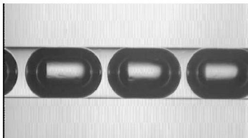
Fig. 1. Concave epoxy microlenses inside glass capillary. Black figures are air bubbles.
