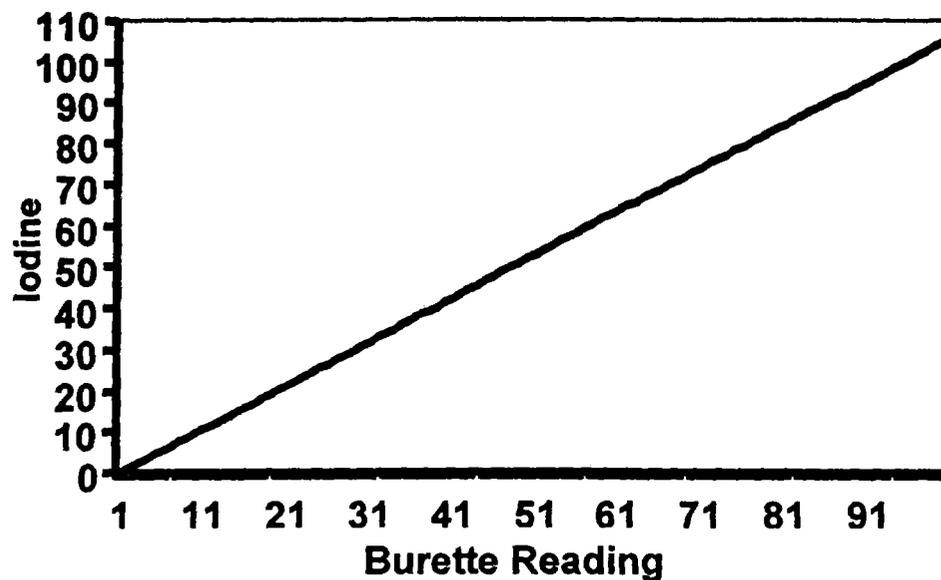
Figure 1: Calibration curve of iodine content versus burette reading
