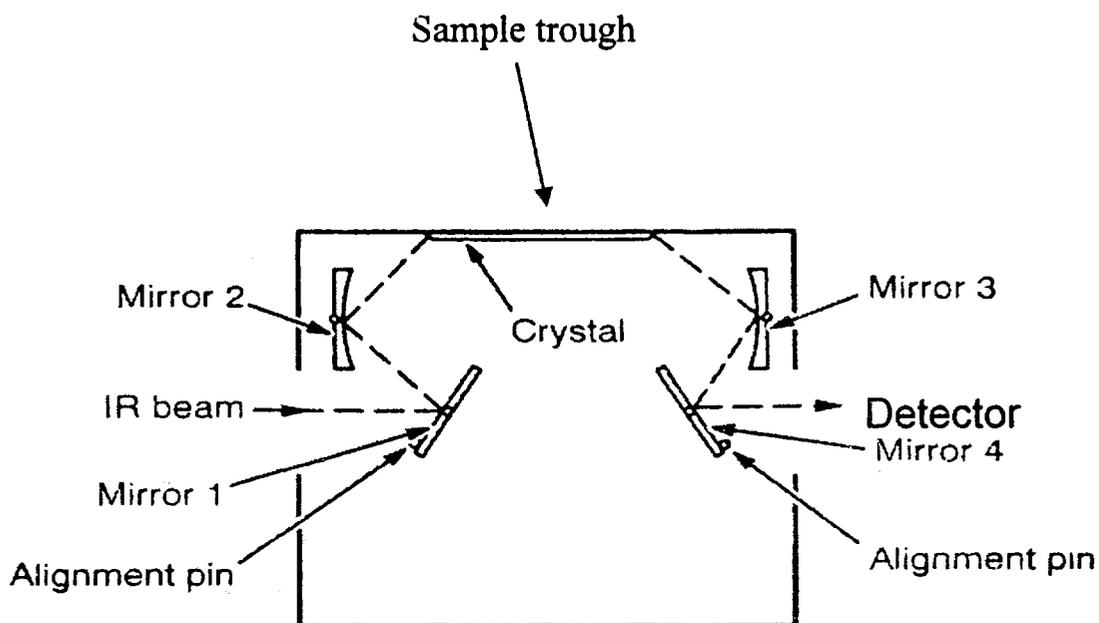
Fig 3: Optical Path of IR Beam in the HATR Sample Trough
