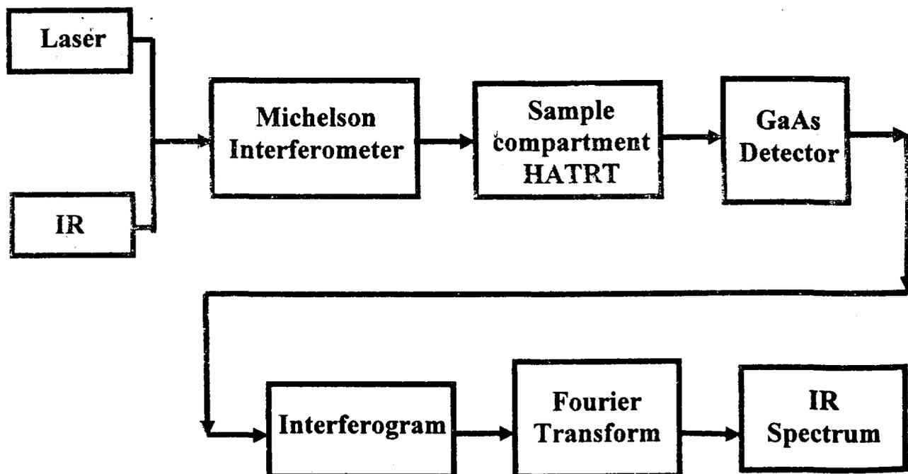
Fig 4: Block diagram of the Vibrational Spectroscopic Method
