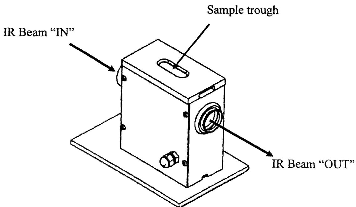
Fig 2: The Horizontal Attenuated Total Reflectance (HATR) with a Sample
