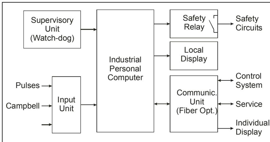
Fig. 5: Block scheme of the OPM channel digital section
