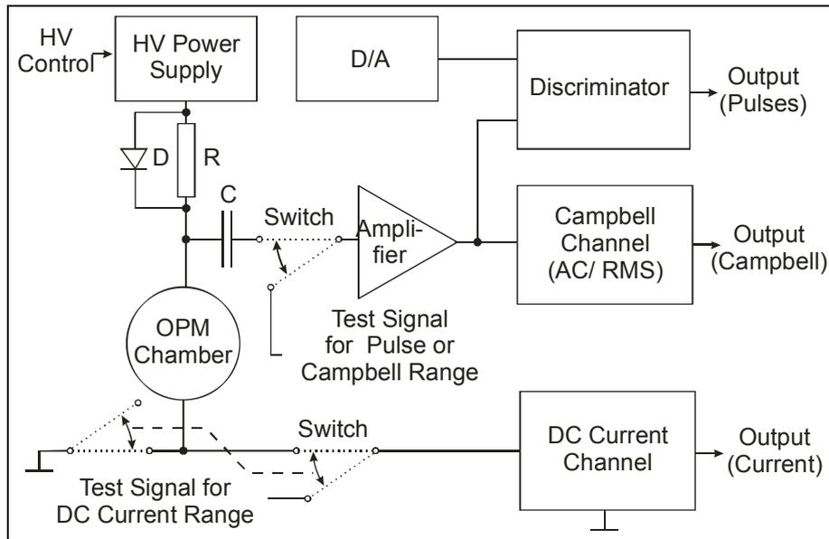
Fig. 4: Block scheme of the OPM channel analog section
