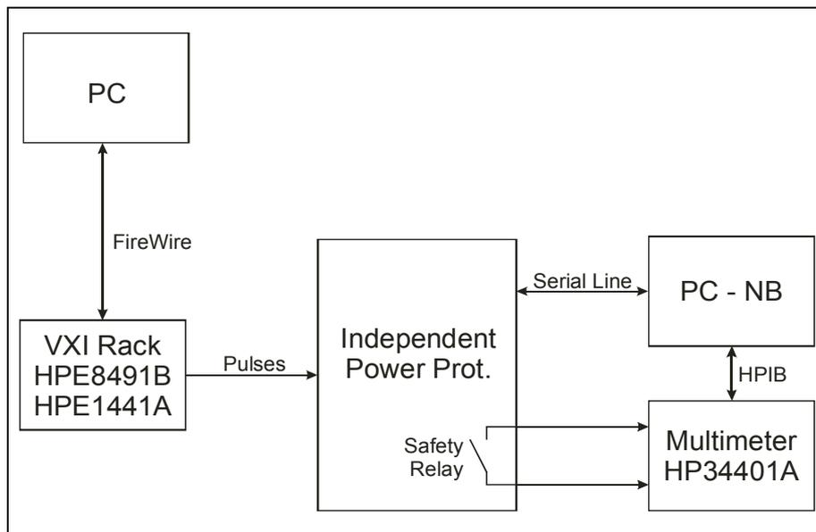
Figure 2: Block diagram of IPP validation tests
