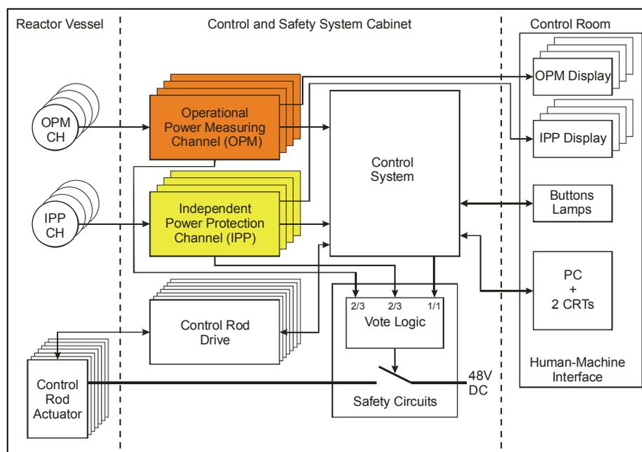
Figure. 1: Block diagram of the upgraded control and safety system
