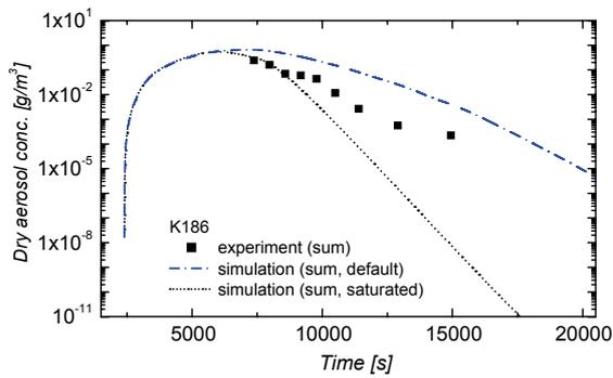
Figure 16: Test K186 - Total dry aerosol mass concentration in test vessel
