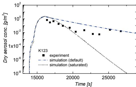
Figure 12: Test K123 - Total dry aerosol mass concentration in test vessel
