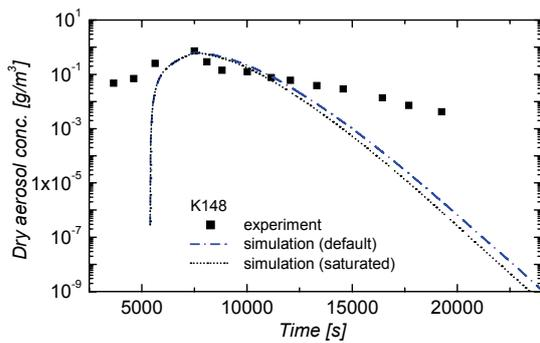
Figure 20: Test K148 - Total dry aerosol mass concentration in test vessel
