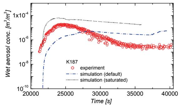
Figure 19: Test K187 - Total wet aerosol volumetric concentration in test vessel
