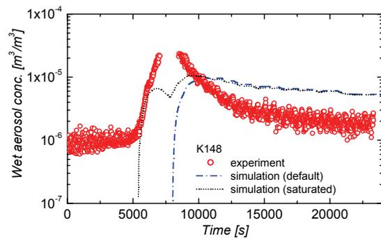
Figure 21: Test K148 - Total wet aerosol volumetric concentration in test vessel
