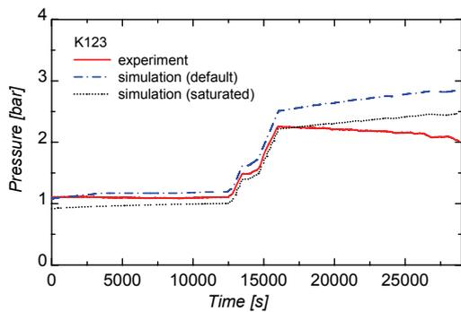
Figure 2: Test K123 - Pressure in test vessel
