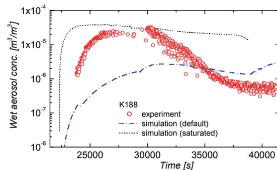
Figure 15: Test K188 - Total wet aerosol volumetric concentration in test vessel
