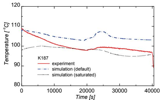
Figure 9: Test K187 - Temperature of test vessel atmosphere
