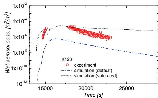
Figure 13: Test K123 - Total wet aerosol volumetric concentration in test vessel
