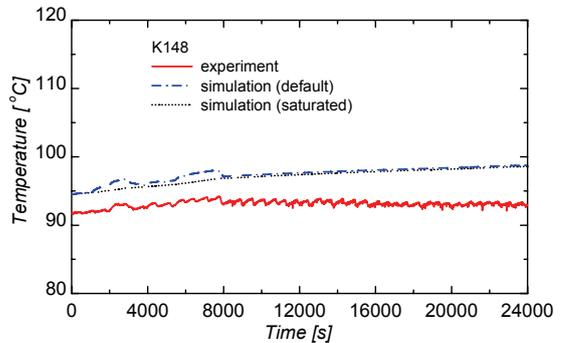
Figure 11: Test K148 - Temperature of test vessel atmosphere
