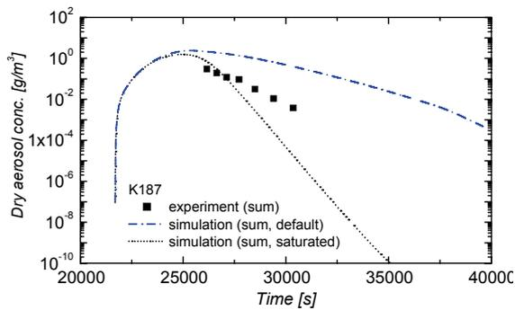
Figure 18: Test K187 - Total dry aerosol mass concentration in test vessel
