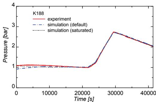
Figure 4: Test K188 - Pressure in test vessel
