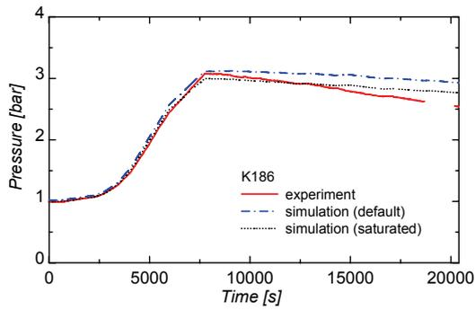
Figure 6: Test K186 - Pressure in test vessel
