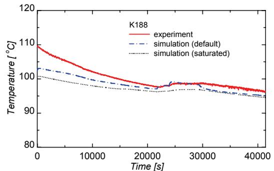
Figure 5: Test K188 - Temperature of test vessel atmosphere
