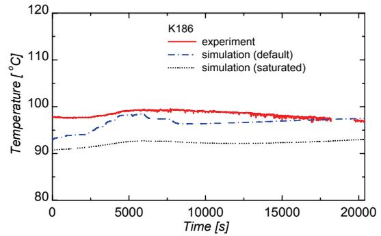
Figure 7: Test K186 - Temperature of test vessel atmosphere
