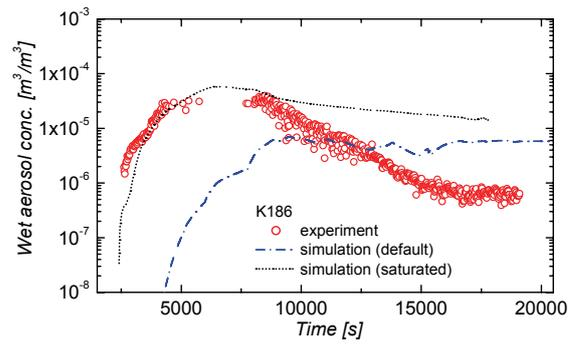
Figure 17: Test K186 - Total wet aerosol volumetric concentration in test vessel
