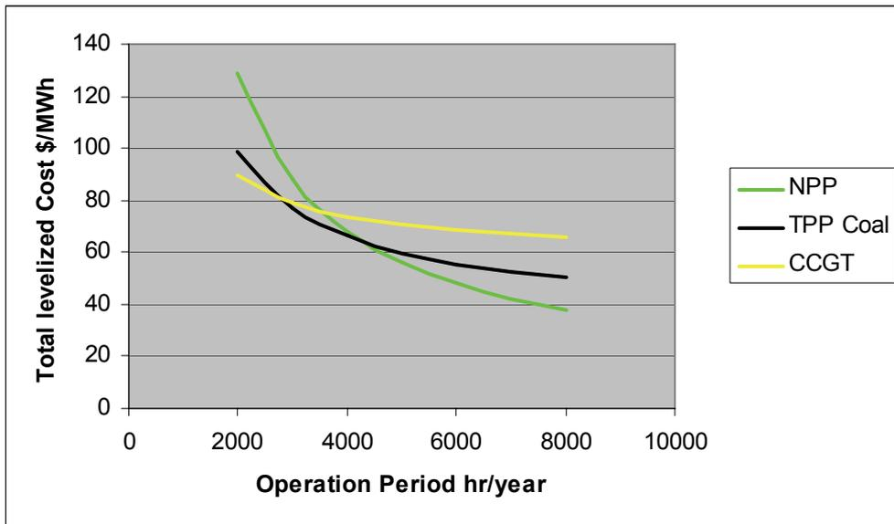
Figure 2: Total Levelized Cost of Electricity for Different Power Plants
