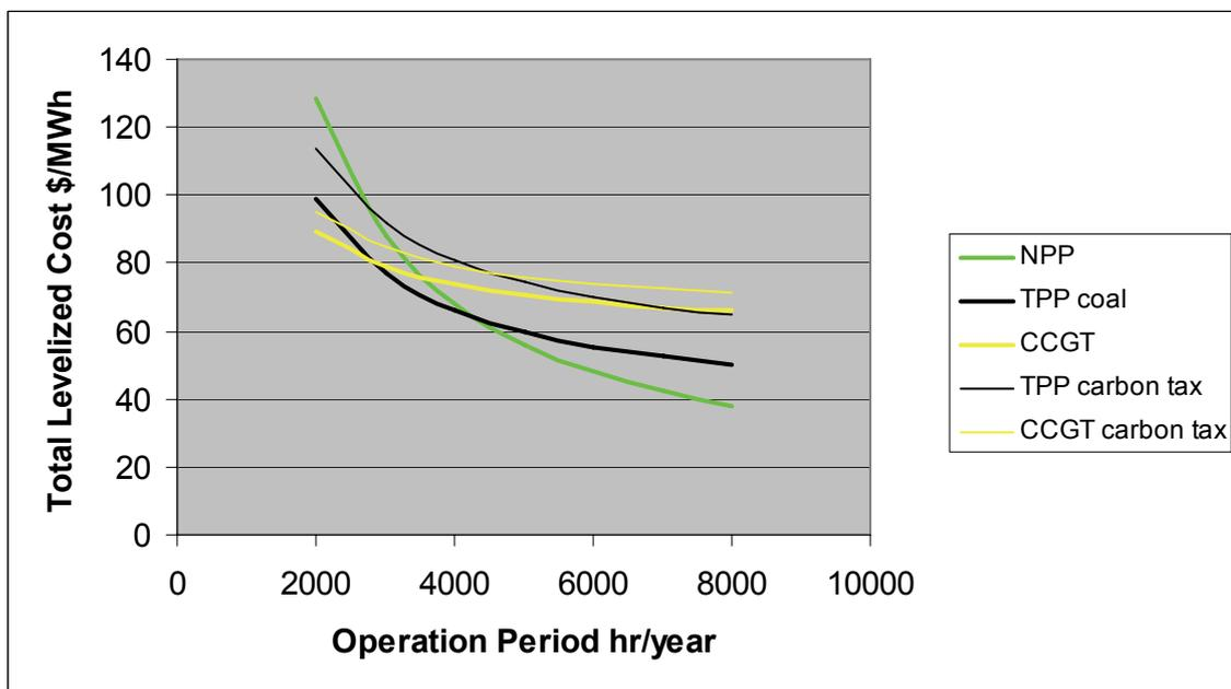
Figure 3: Total Levelized Cost of Electricity-Carbon Taxes included (1.2\$/GJ-coal, 0.6\$/GJ-gas)
