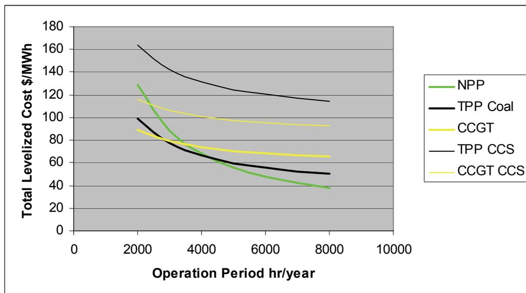
Figure 4: Total Levelized Cost-the Cost of CCS included (50\$/tonne CO<sub>2</sub>)
