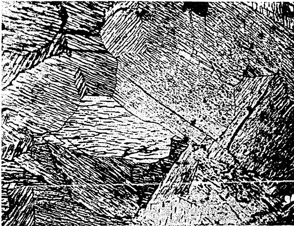
Fig. I - Micrograph of uranium monocarbide X 300 -
