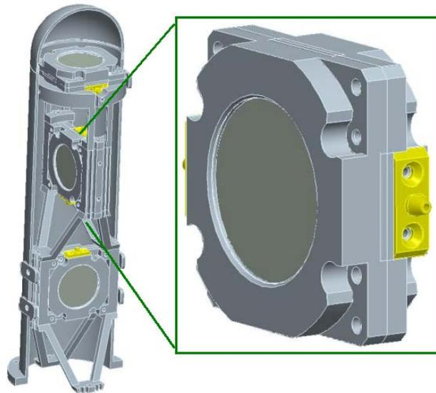
**Figure 3: The arrangement of the three telescopes (x, y and z axis) in the external unit**
