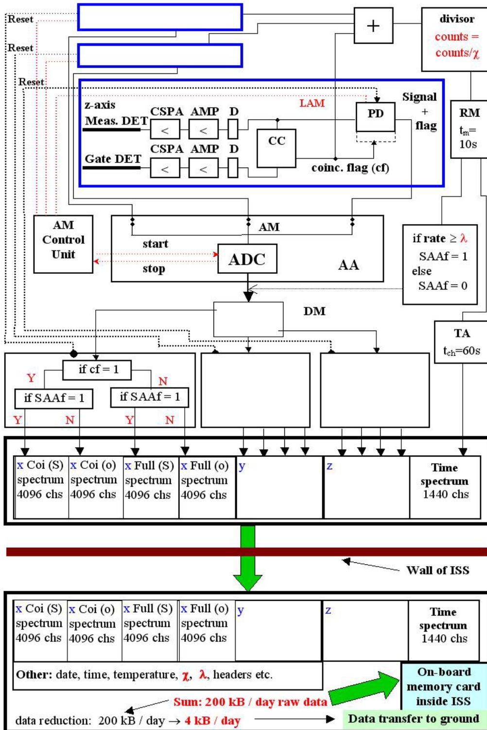
Figure 4: Simplified block diagram of Tritel three-dimensional silicon detector telescope
