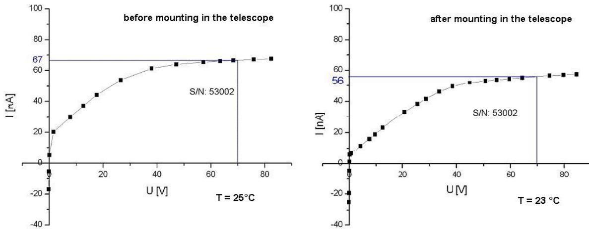
Figure 6: The reverse current of the Canberra fully depleted silicon detector as a function of the bias
