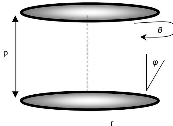
Figure 2: The main geometric parameters of the telescope ( $r$  is the radius of the detector and  $p$  is the distance between the detector chips) [3]
