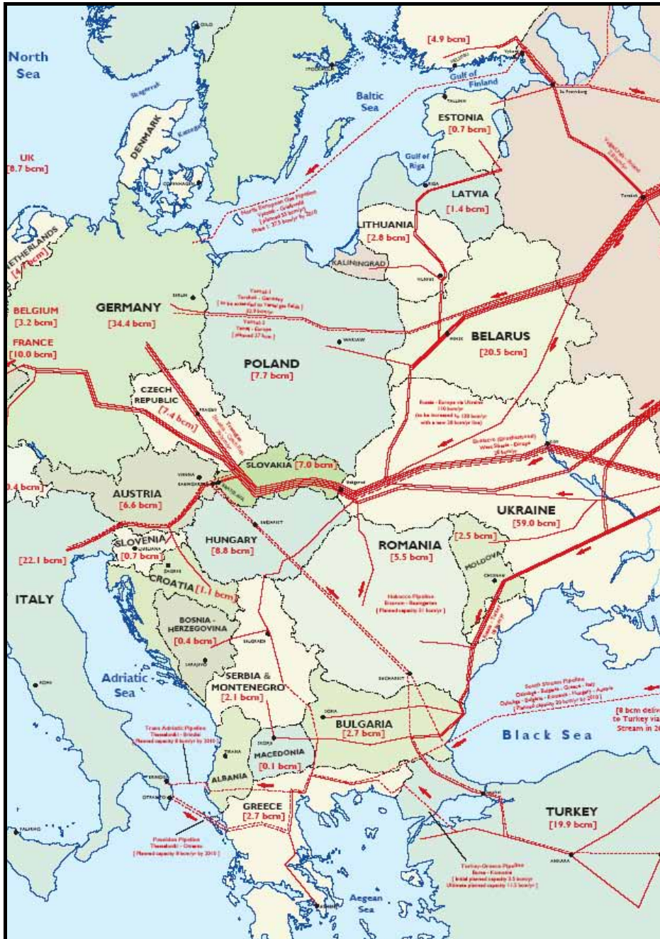
Figure 5: Gas pipelines from the FSU to Europe
