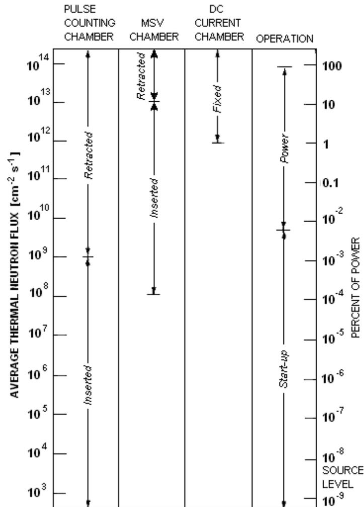
Fig. 5.2: Ranges of in-core fission chambers
