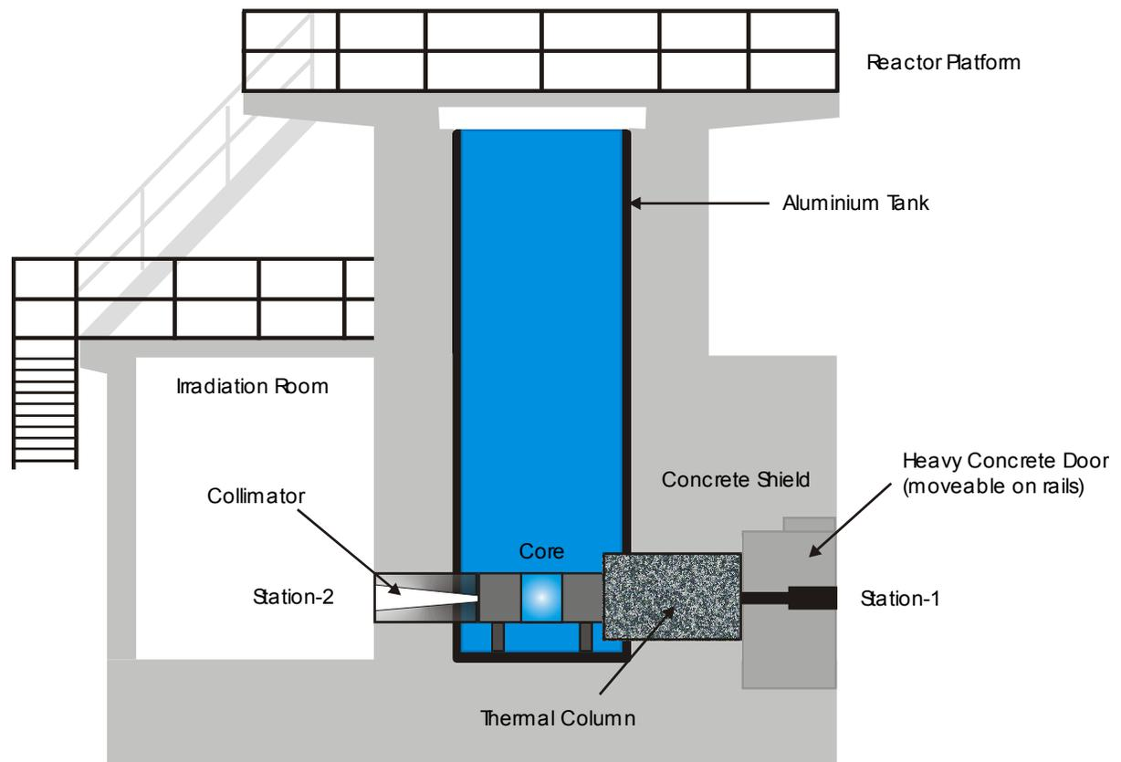
Fig. 8.1: Vertical cross section
