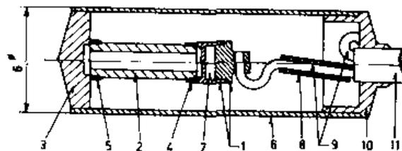
Fig. A.2: Neutron sensitive thermocouple model
