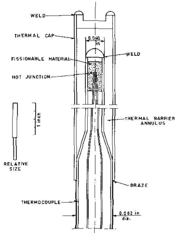
Fig. A.1: Neutron sensitive thermocouple model 1
