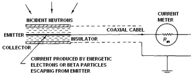
Fig. 6.2: Self powered neutron detector
