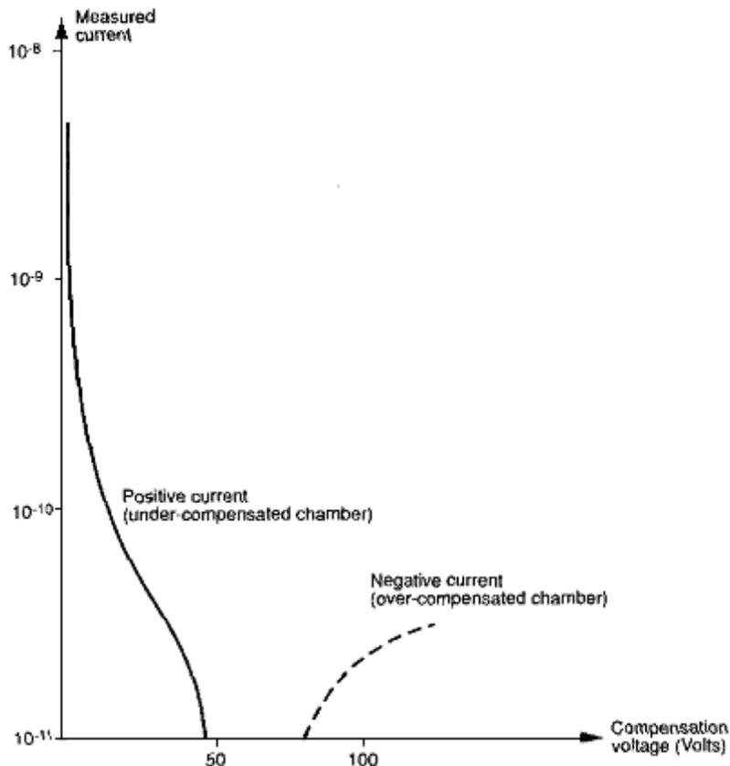
Fig. 4.3: Typical plot of a compensation curve
