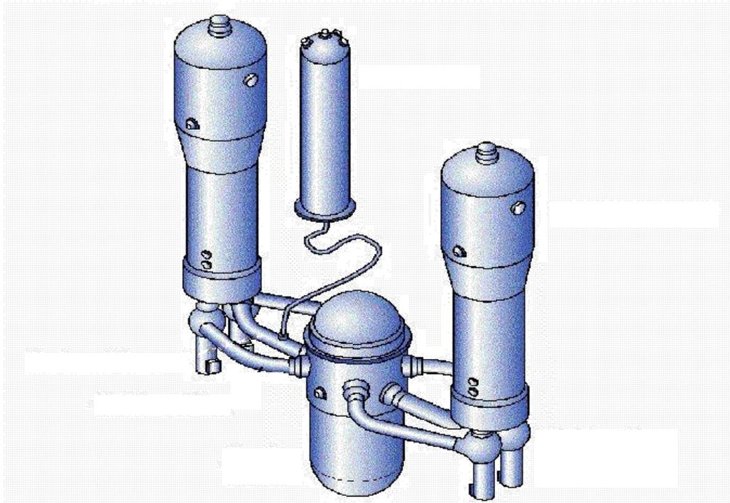
Figure 7.1 - A typical 600 MWe Pressurized Water Reactor NPP
