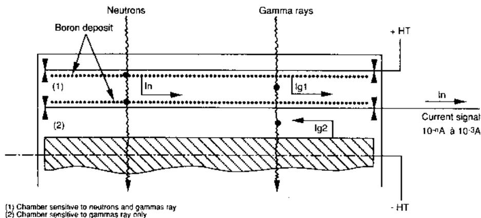
Fig. 4.2: Compensated ionisation chamber mimic diagram
