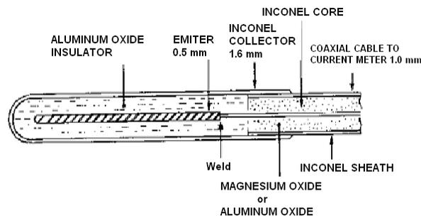
Fig. 6.1: Self powered neutron detector
