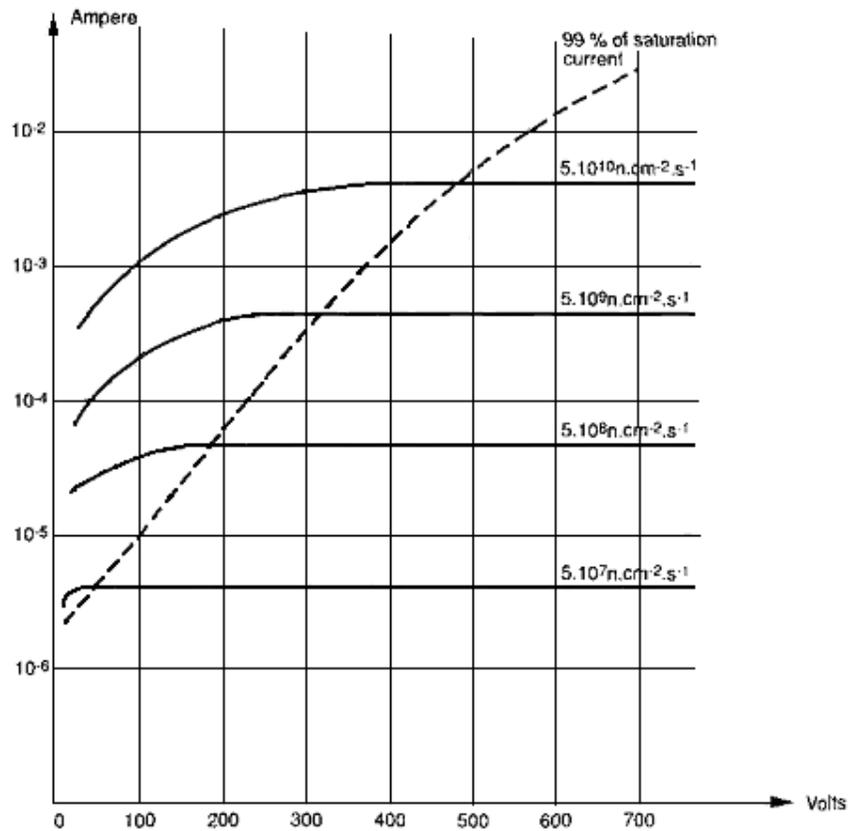
Fig. 4.4: Saturation curve array
