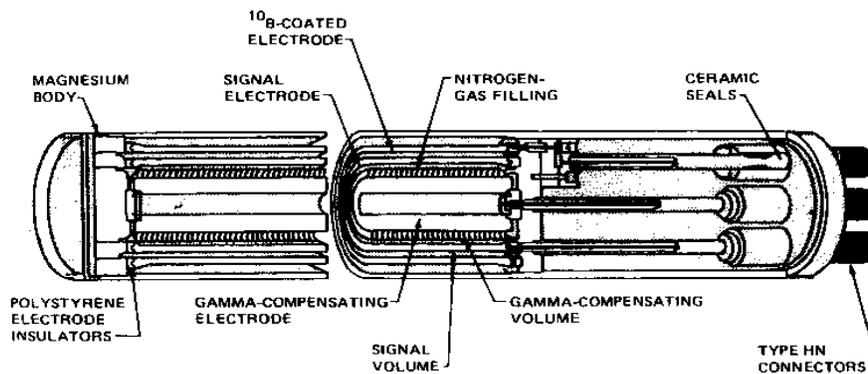
Fig. 4.1: Cross section through a CIC
