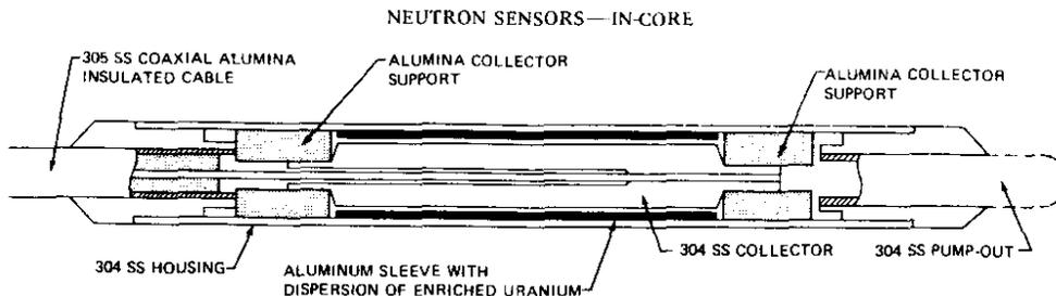
Fig. 5.1 Cross section through miniature in-core fission chamber
