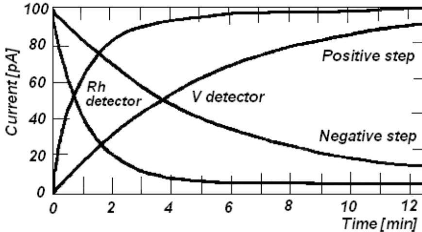
Fig. 6.3: SPND response to step change in neutron flux
