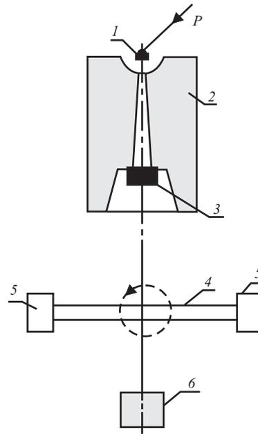
Fig. 3. Scheme of Italian experiment. 1 — lithium target; 2 — shielding; 3 — scatterer; 4 — position-sensitive spectrometer; 5 — photomultiplier; 6 — neutron direct beam detector
