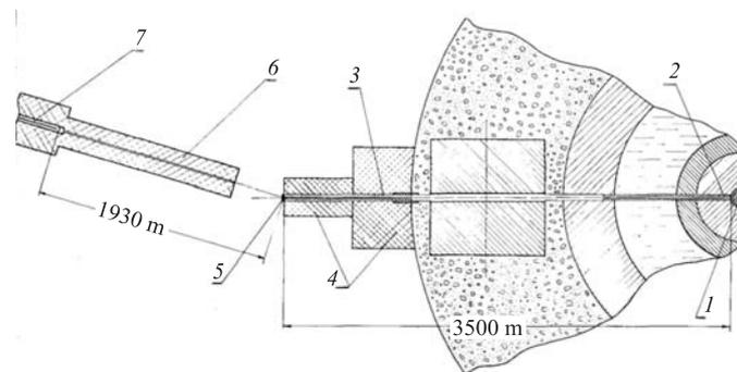
Fig. 1. Apparatus for measurements of the small-angle neutron scattering. 1 — reactor active zone; 2, 3 — steel collimators; 4, 6 — paraffin shielding; 5 — target; 7 — detector
