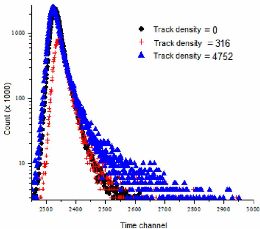
**Fig. 3.** Typical lifetime spectra for CR-39
