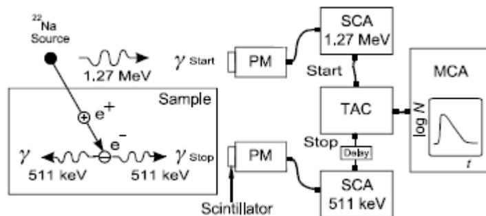
Fig. 1. Principle of basic lifetime spectroscopy
