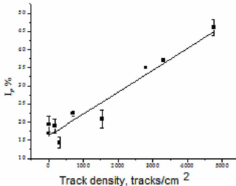
Fig. 4. The linear dependence  $I_3$  – track density for CR-39
