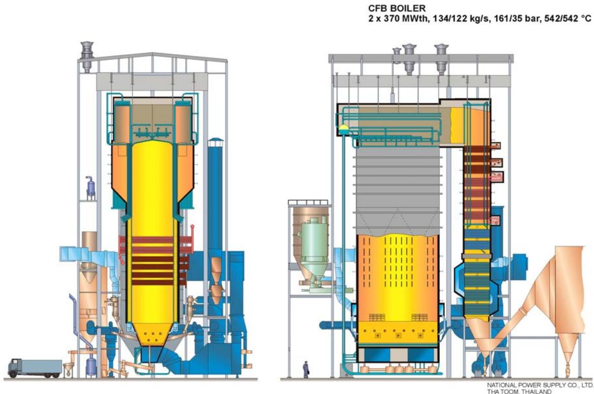
*Figure 4: The cross section of the Compact CFB Boilers.
