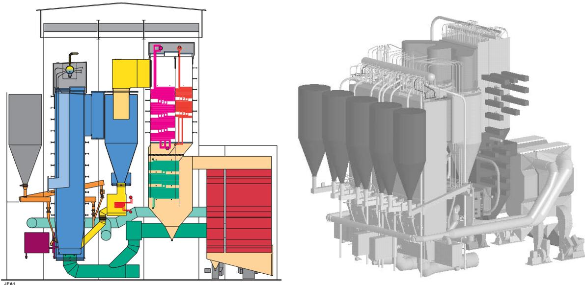
Figure 6: The 300 MWe class CFB boiler designed to fire 100% bituminous coal and 100% high sulfur petroleum coke (cross-section and 3D model)
