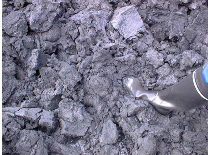
Figure 8: Coal slurry requires specific handling equipment but its cost effective energy source when fired in CFB boilers
