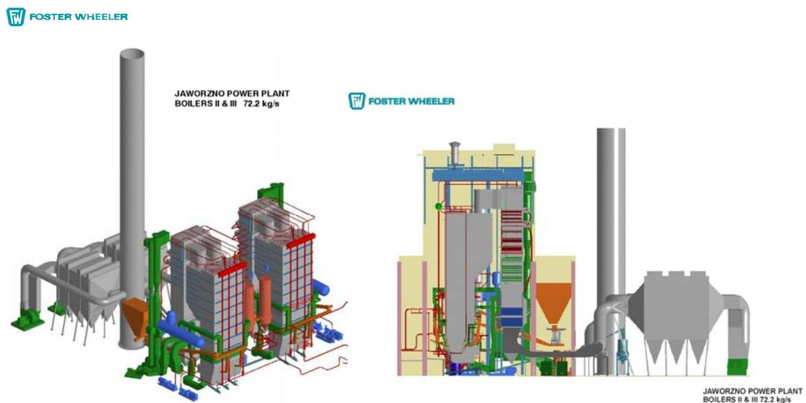
Figure 7: Jaworzno CFB boiler designed to fire 100% Bituminous Coal and mixture of Bituminous Coal and Coal Slurry (cross-section and 3D model)
