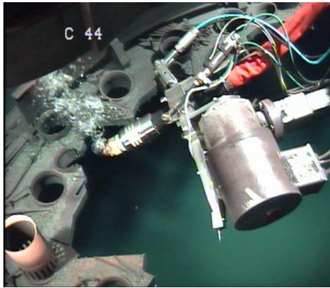
Fig.1 Plasma nozzle mounted on the endeffector of the manipulator system
