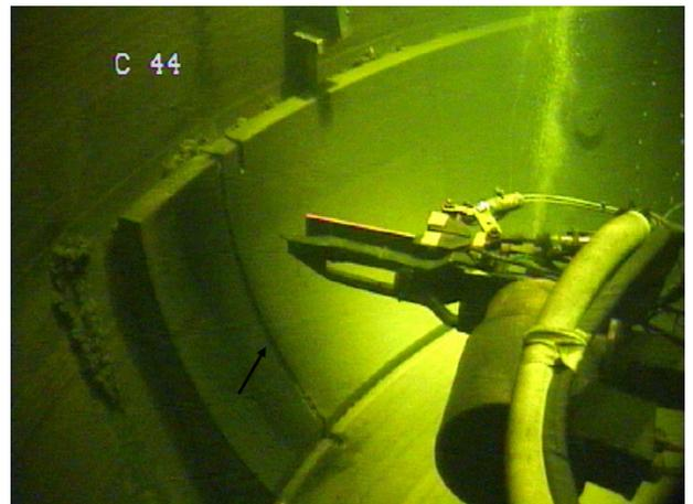
Fig.5 CAMC-assembly with electrode and at its left the teaching finger in front of the lower thermal shield wall
