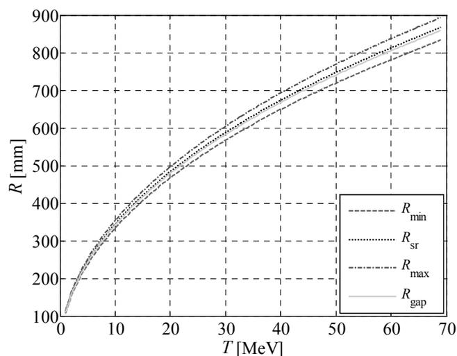
Fig.1. The dependence of the SEO mean,  $R_{sr}$ , minimal,  $R_{min}$ , and maximal,  $R_{max}$ , radius on the ion kinetic energy. Also shown is the influence of the test ion kinetic energy on the ion radial position within the acceleration gap,  $R_{gap}$ . The test ion is  $H^-$  with the extraction energy of 65 MeV at the extraction radius  $R_{sr} = 84$  cm.
