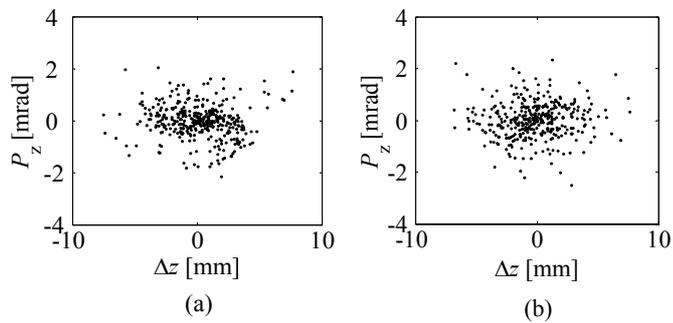
Fig.8. The vertical emittances for (a) the optimal initial conditions, and (b) the non-optimal initial conditions
