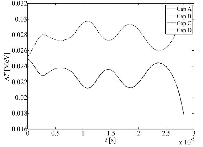
Fig.4. The central ion energy gain within gaps for the optimal initial conditions
