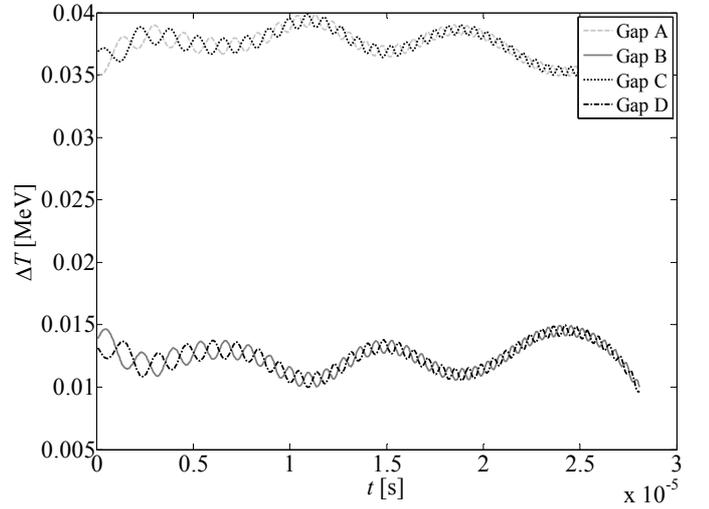
Fig.5. The central ion energy gain within gaps for the non-optimal initial conditions
