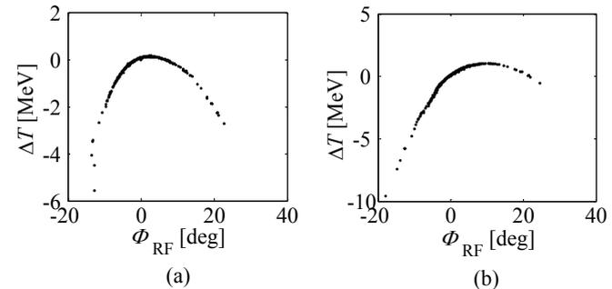
Fig.9. The longitudinal emittances for (a) the optimal initial conditions, and (b) the non-optimal initial conditions
