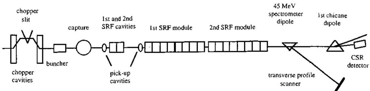
Fig. 2 Block diagram of CEBA injector layout
