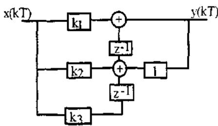
Figure 1. Direct implementation of a PID controller
