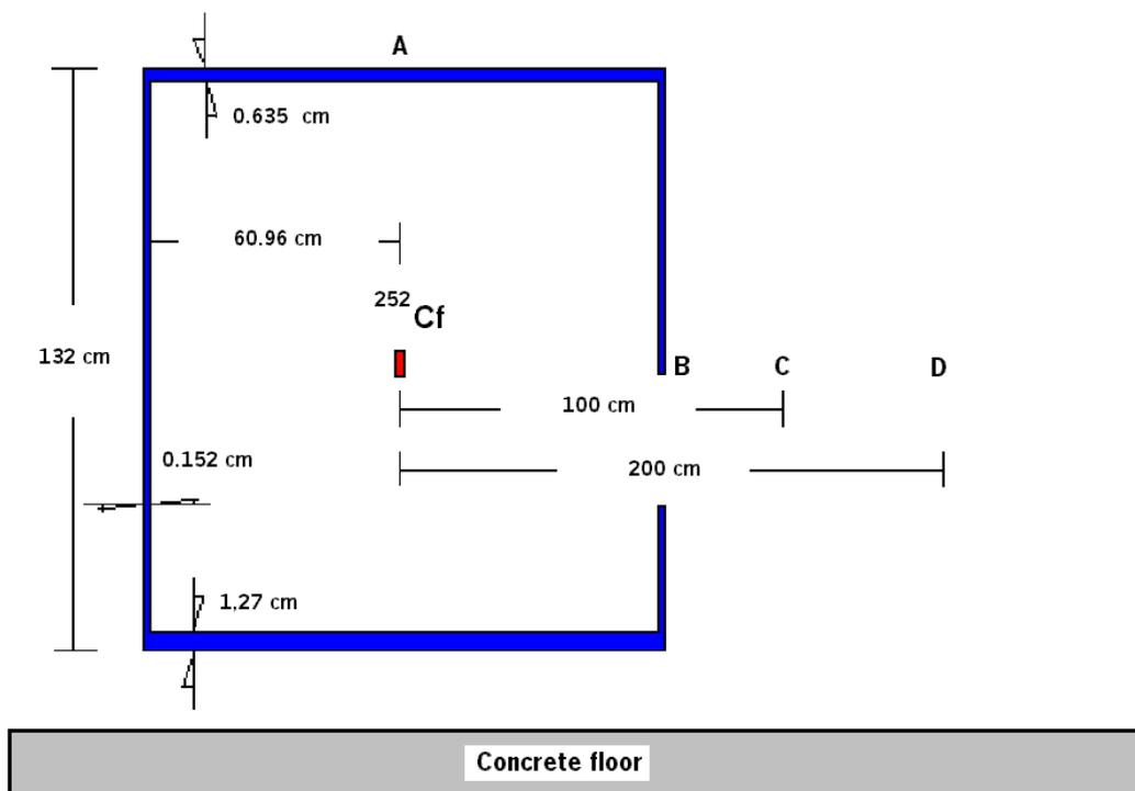
Figure 4.- WEP shield structure modeled in the Monte Carlo calculations.
