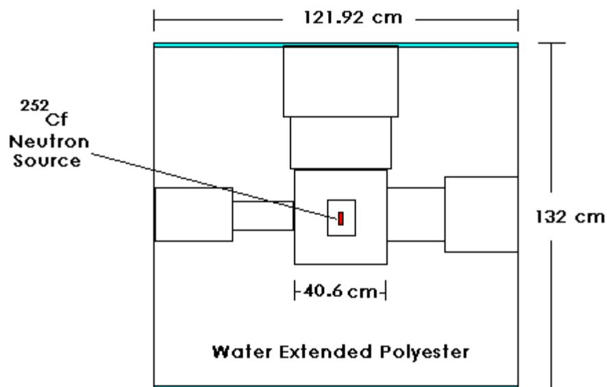
Figure 1.- Nuclear Engineering Teaching Laboratory WEP neutron shielding.
