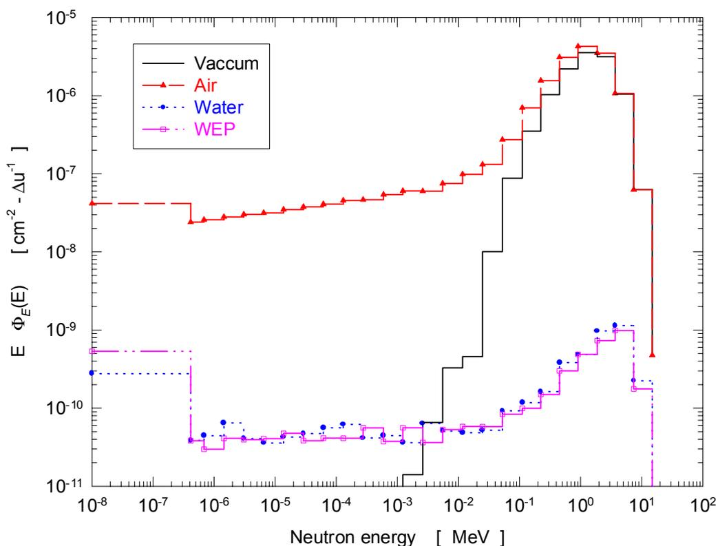
Figure 5.-  $^{252}\text{Cf}$  lethargy neutron spectrum in vacuum, air, water and WEP
