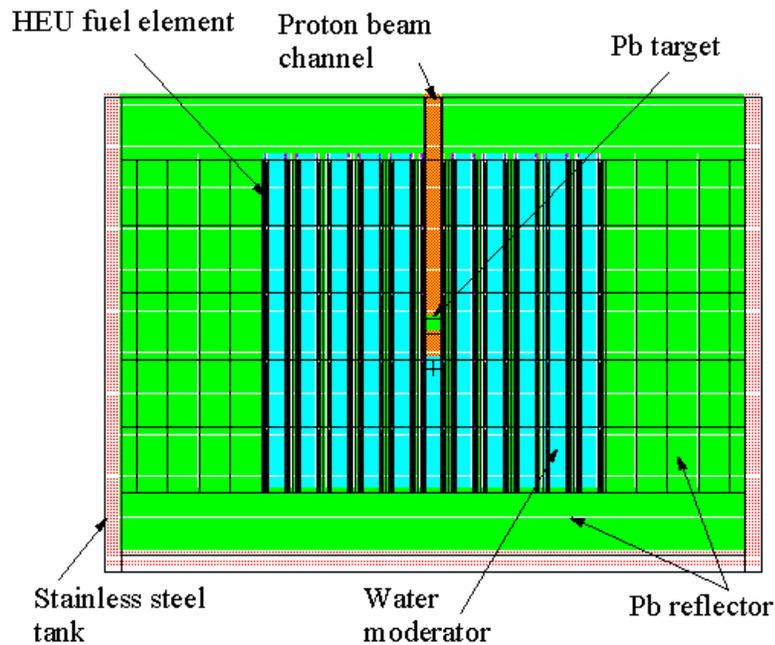
Figure 4. Vertical cross-section (at the target plane) of the proposed ADS
