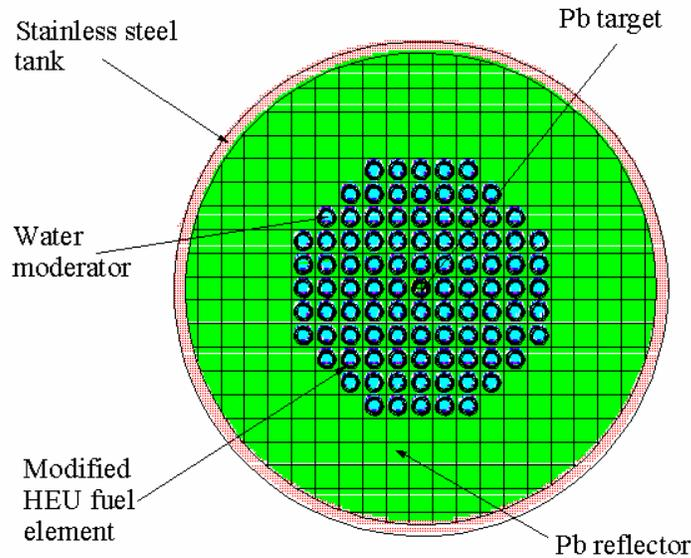
Figure 3. Horizontal cross-section (at the target plane) of the proposed ADS
