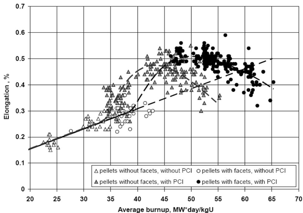
Fig. 1. Change of the Fuel Rod Length as the Function of Average Burnup [5].
