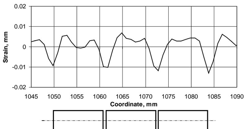
Fig. 2. Changes of the Cladding Diameter along the Height [6].
