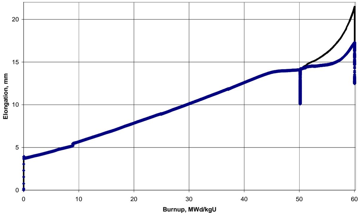
Fig. 3. Change of the Fuel Rod Length versus Burnup.
