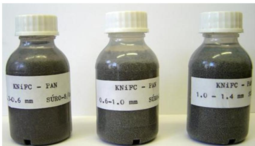
Fig.3 Different size of KNiFC-PAN sorbent
