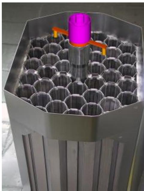
Fig.8 Detector on the head of storage container
