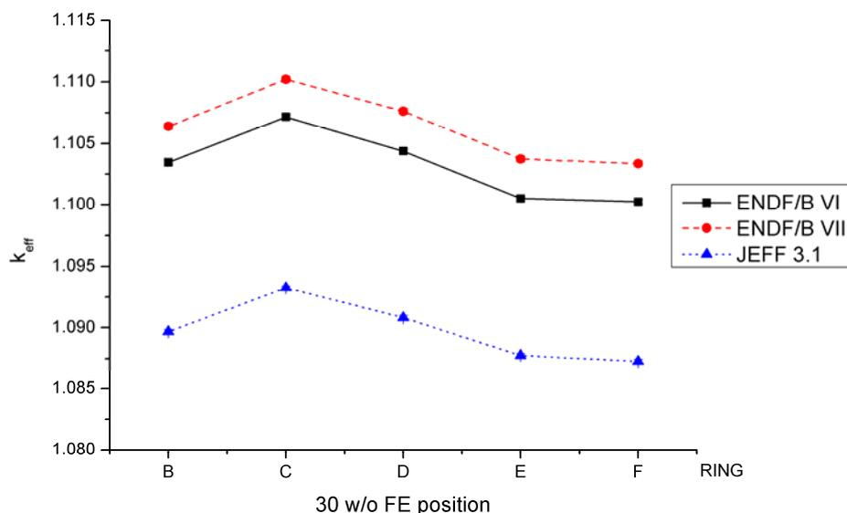
Figure 5.  $k_{\text{eff}}$  as a function of 30 w/o FEs location in mixed core filled with 8.5 w/o fuel. Note that in each case six 30 w/o FEs are inserted in individual ring.
