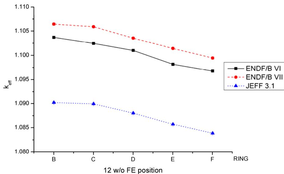
Figure 3.  $k_{\text{eff}}$  as a function of 12 w/o FEs location in mixed core filled with 8.5 w/o fuel. Note that in each case six 12 w/o FEs are inserted in individual ring.
