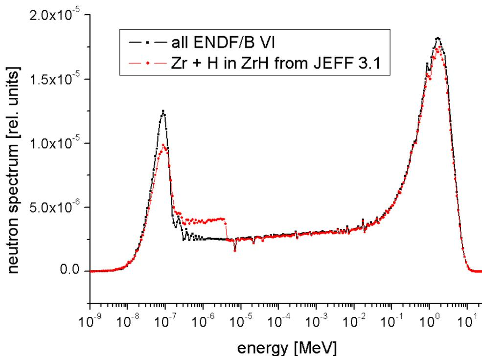
Figure 2. Neutron spectrum in the fuel calculated with MCNP. In the first case (all ENDF/B VI) neutron spectrum was calculated taking all cross sections from ENDF/B VI and in second case Zr and H in ZrH cross sections were taken from JEFF 3.1 [4], other cross sections were from ENDF/B-VI.
