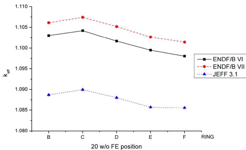
Figure 4.  $k_{\text{eff}}$  as a function of 20 w/o FEs location in mixed core filled with 8.5 w/o fuel. Note that in each case six 20 w/o FEs are inserted in individual ring.
