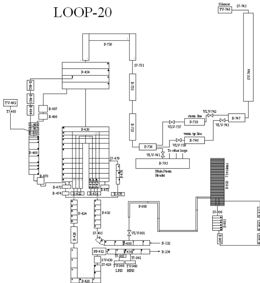
Figure 3: RELAP5 noding diagram of PKL III loop 2, pressurizer and secondary system
