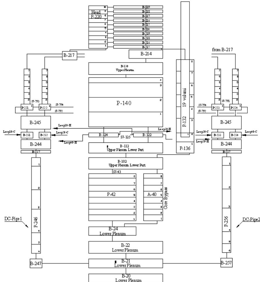
Figure 2: RELAP5 noding diagram of PKL III vessel
