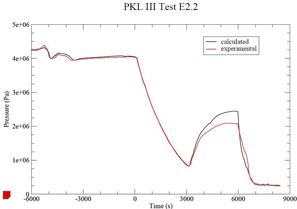
Figure 5: E2.2 experiment and analysis results for pressurizer pressure
