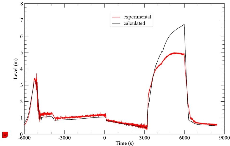
Figure 6: E2.2 experiment and analysis results for pressurizer collapsed level
