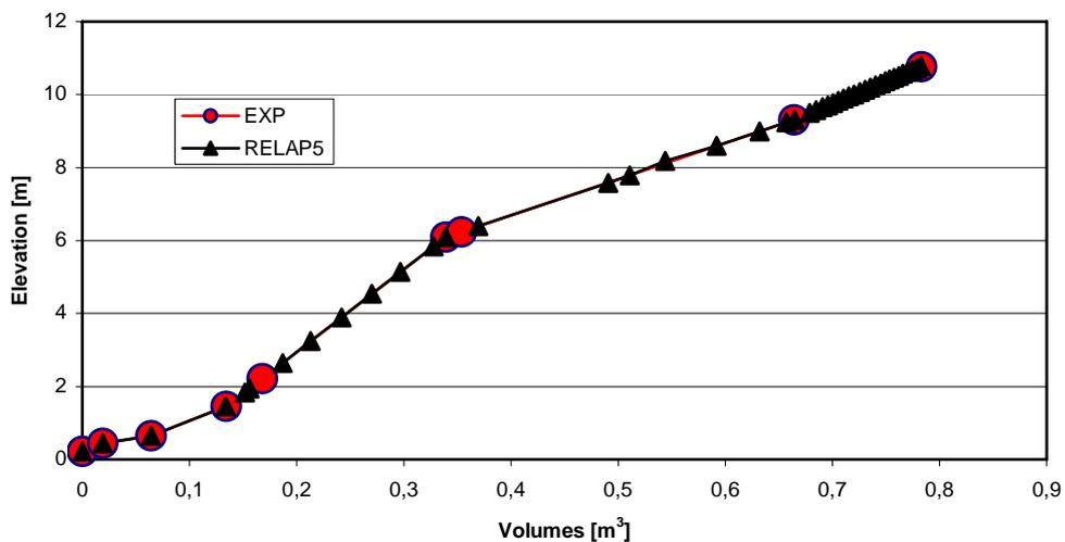
Figure 4: Comparison between experimental and adopted values for the elevations vs volumes distribution in PKL III rod bundle vessel
