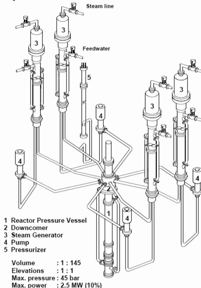
Figure 1: PKL III Test Facility
