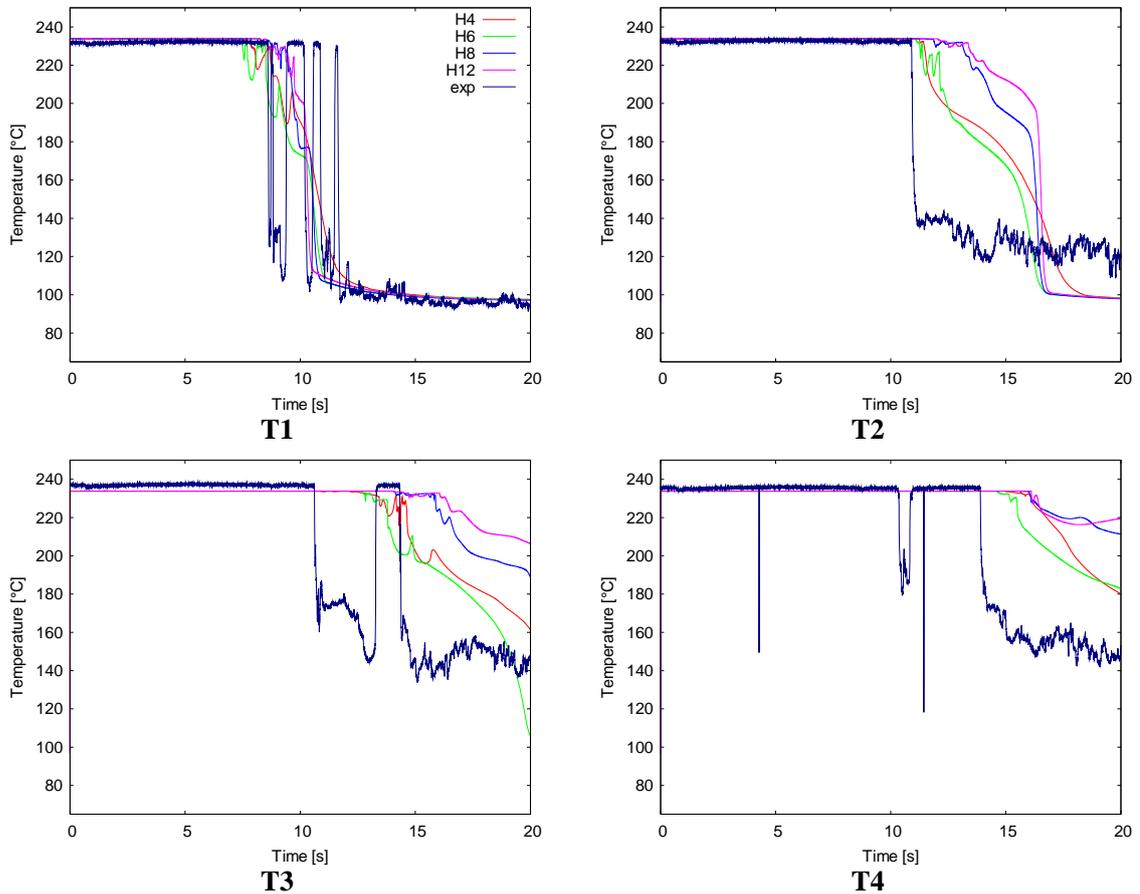
Figure 4: Local temperatures in numerical simulations of whole domain on different meshes and experiment at 4 measurement points.
