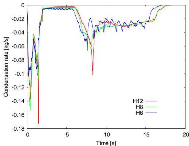
Figure 5: Condensation rate in numerical simulations of whole domain calculated on different meshes.
