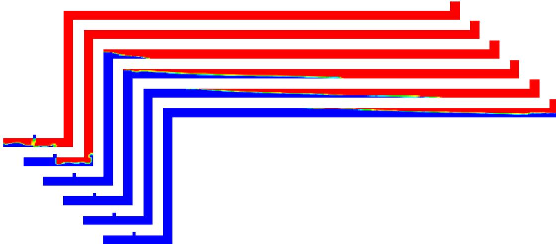
Figure 6: Volume fraction in simulation of whole domain at different time steps (0.25 s, 1 s, 6s, 8 s, 10 s, 14 s).
