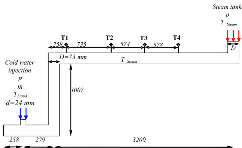
Figure 1: Numerical domain with boundary conditions and local measurements of temperature ( $p=30$  bar,  $T_{Liquid}=97^\circ\text{C}$ ,  $T_{Steam}=234^\circ\text{C}$ ,  $\dot{m}=1$  kg/s).
