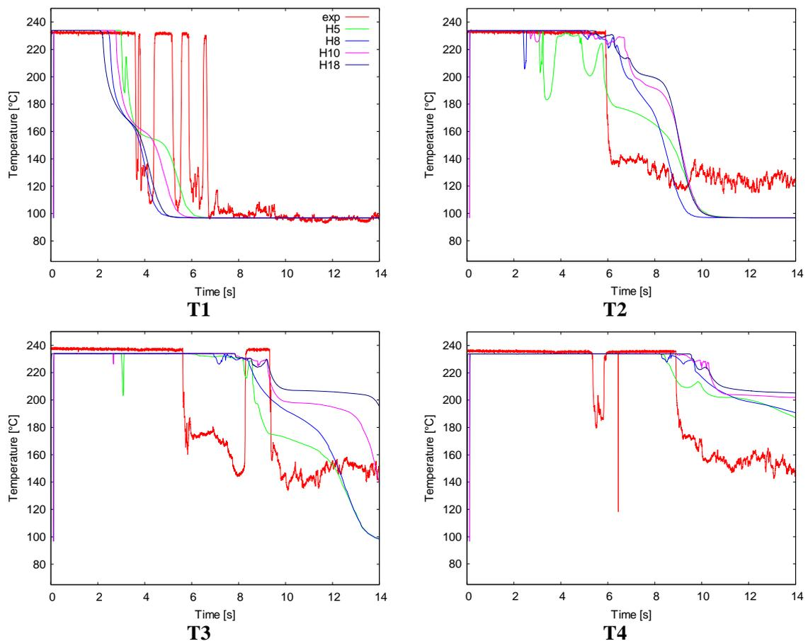
Figure 2: Local temperatures in simplified numerical simulations on different meshes and experiment at 4 measurement points.
