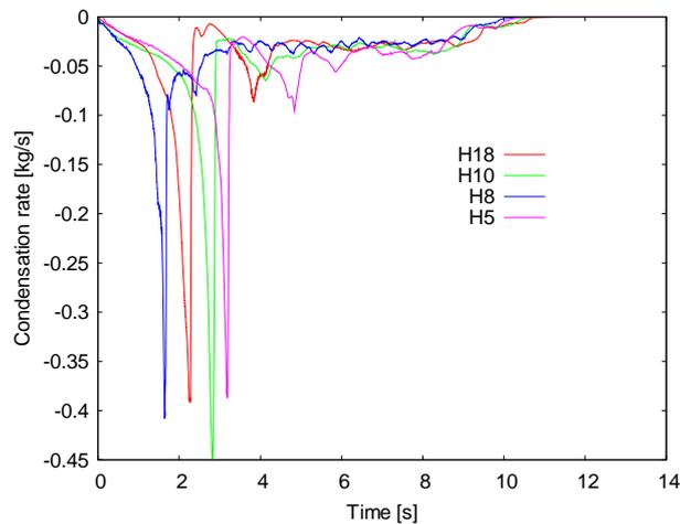
Figure 3: Condensation rate (integral) in simplified numerical simulations calculated on different meshes.
