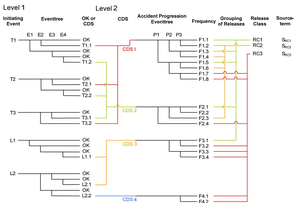
Figure 1: Schematic of the integrated approach for the L1 to L2 transition. The core damage sequences are grouped to core damage states (CDS) and passed on to the accident progression event trees (APET). The endpoints of the APET are grouped into release classes for which frequencies and source terms are calculated.
