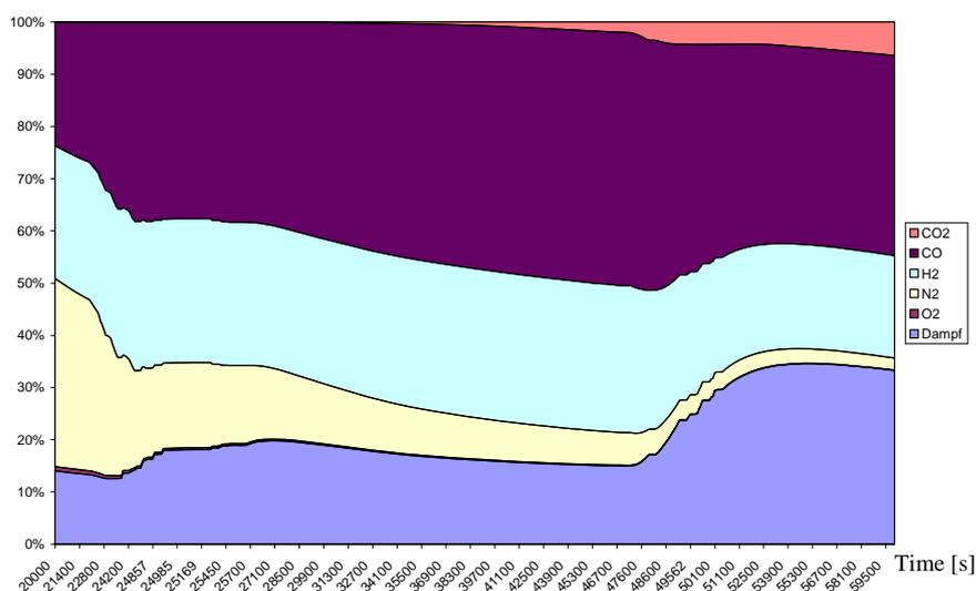
Figure 2: Composition of the atmosphere in the wetwell. Even during the second venting cycle (13 h after the initiating event) the peak fraction of condensable gases (“Dampf”) is low enough to prevent containment under-pressure issues. (After 6 h the vent was opened for the first time.)
