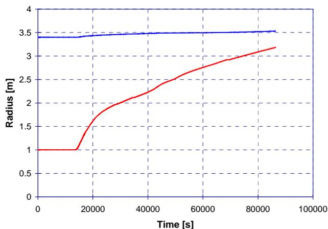
Figure 3: Radial ablation of the lower portion of the CRD room and the containment sump by molten corium for a total loss of injection to the RPV.
