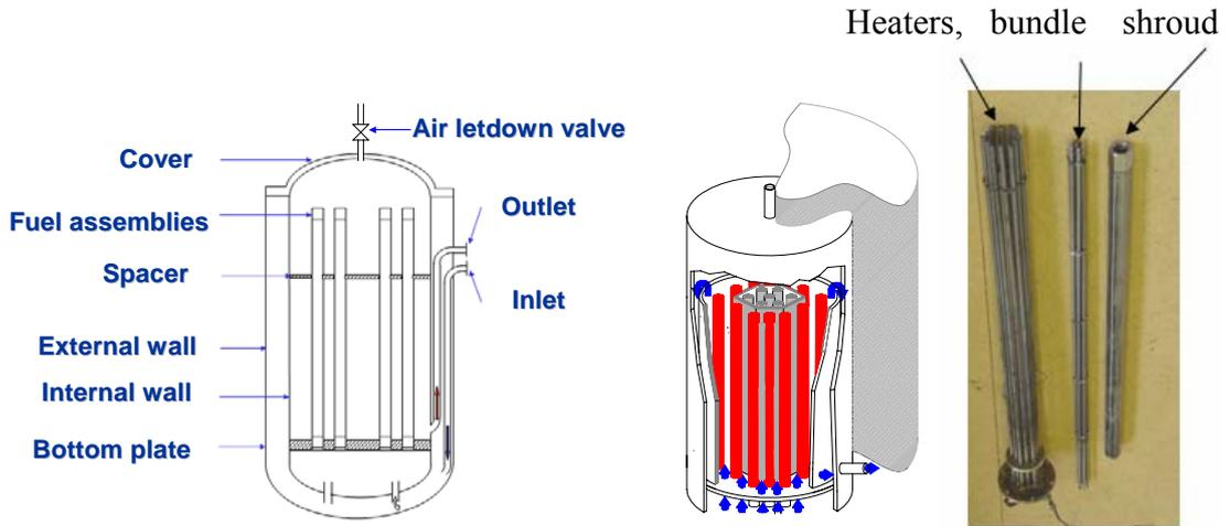
Fig. 2. Design of the cleaning tank, scheme of the CODEX-CT test section and picture of the bundle
