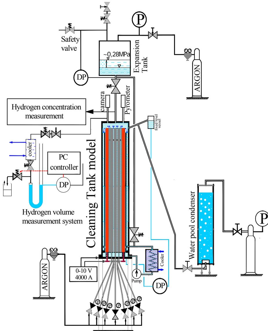
Fig. 3 Main components of the CODEX-CT facility
