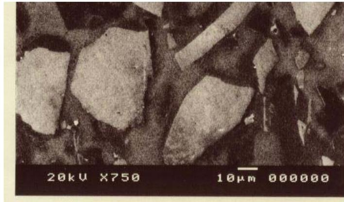
Fig. 3. SEM section for a printed part dipped in liquid Si,750x .
