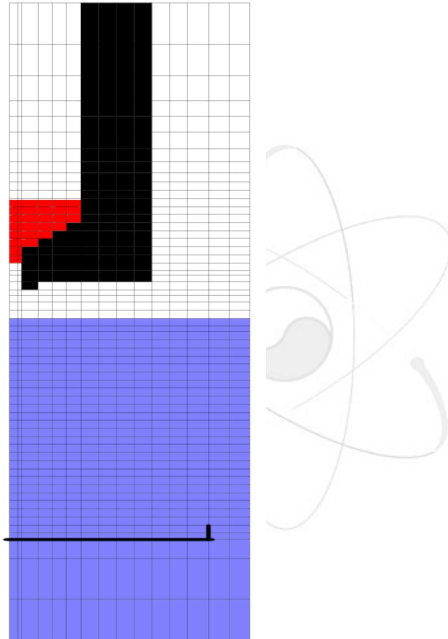
**Figure 19:** Calculation region for PREMIX simulation with meshing (thin black lines), no-flow zones (black areas), debris catcher (thick black lines), and the initial positions of water (blue/light grey area) and melt (red/dark grey area). The scales are different in the two directions.
