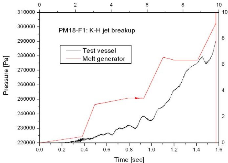
**Figure 21:** Gas pressure in the test vessel, calculated with the Kelvin-Helmholtz jet break-up model. The calculation is valid until blow-through occurs at 1.537 sec. The pressure in the melt generator is prescribed until 1.572 sec, i.e. except for the extremely fast changes in the end.
