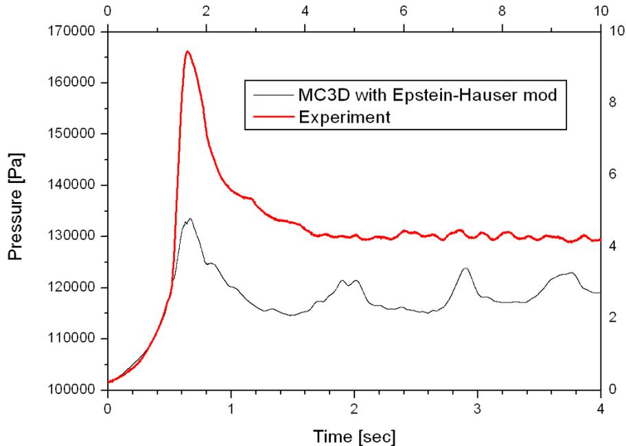
**Figure 14:** Comparison of experimental and calculated pressure development in the gas space of the test vessel when using the Epstein-Hauser modified film boiling model. All other parameters are identical to the base case.
