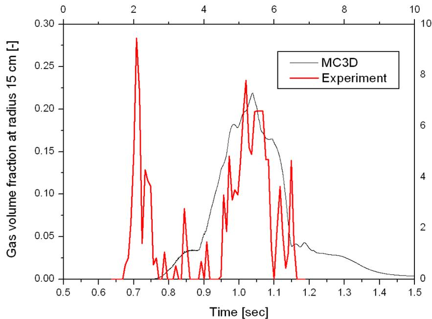
**Figure 8:** Comparison of experimental and calculated void histories at 15 cm radius. Mind the different scale on the ordinate.
