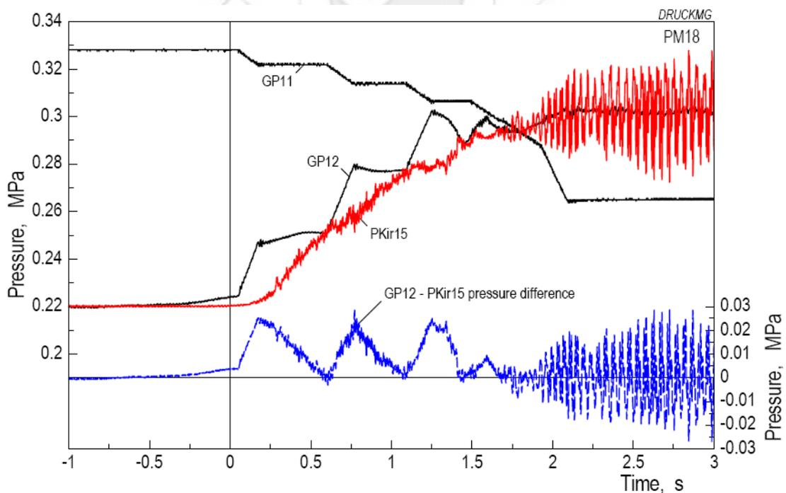
**Figure18:** Pressures controlling the melt release in PM18 (from Ref. 4)
