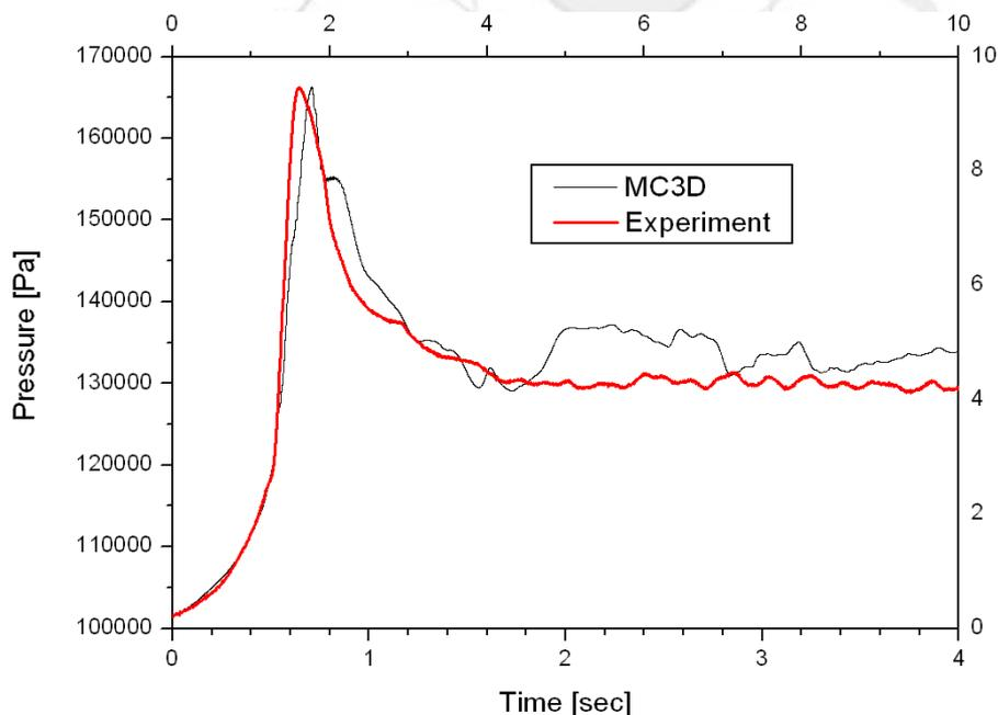
**Figure 6:** Comparison of experimental and calculated pressure development in the gas space of the test vessel.
