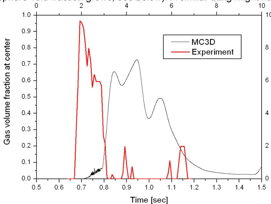
**Figure 7:** Comparison of experimental and calculated void histories
