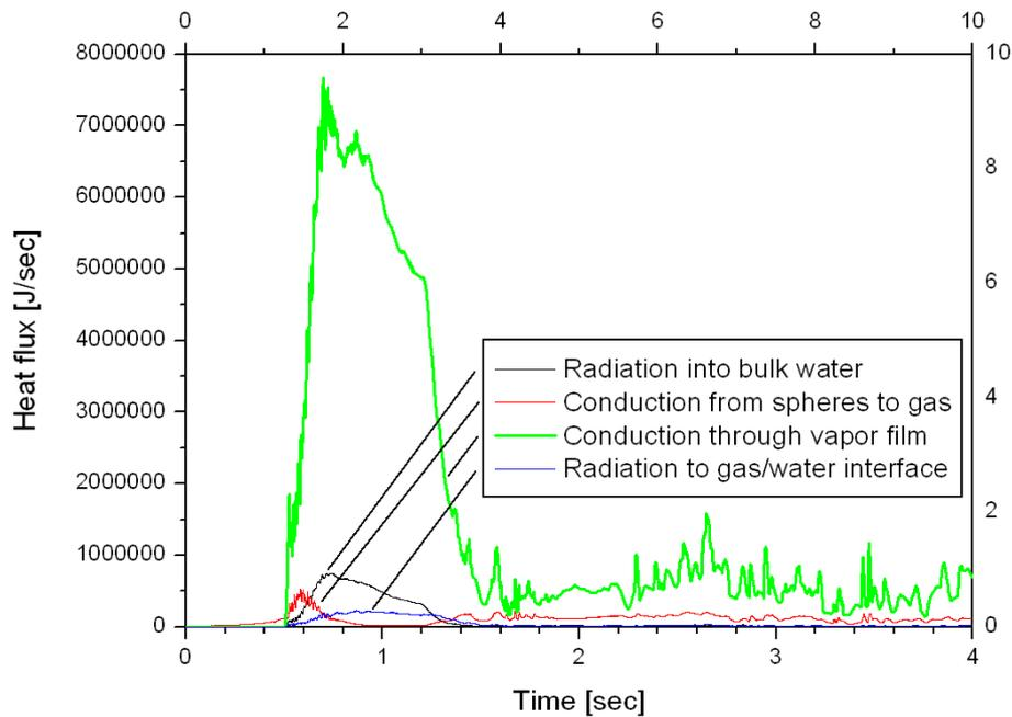
**Figure 11:** Comparison of the most important heat fluxes, integrated over the whole calculation domain.
