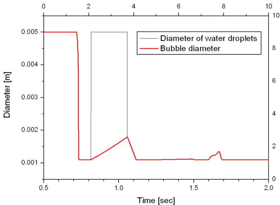
**Figure 16:** Diameters of water drops and bubbles in the cell from which the central void is taken. Minimum bubble diameter: 1.10 mm.
