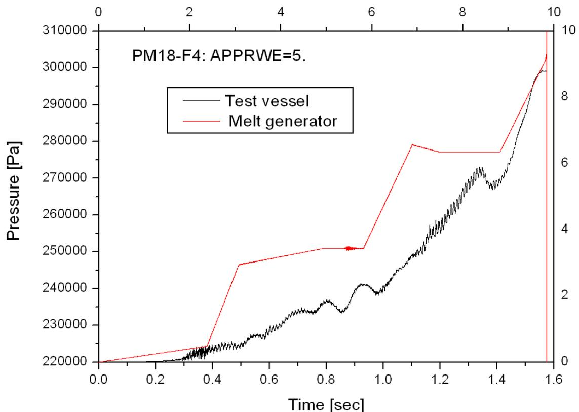
**Figure 22:** Gas pressure in the test vessel, calculated with the Kelvin-Helmholtz jet break-up model. The calculation is valid until blow-through occurs at 1.575 sec.
