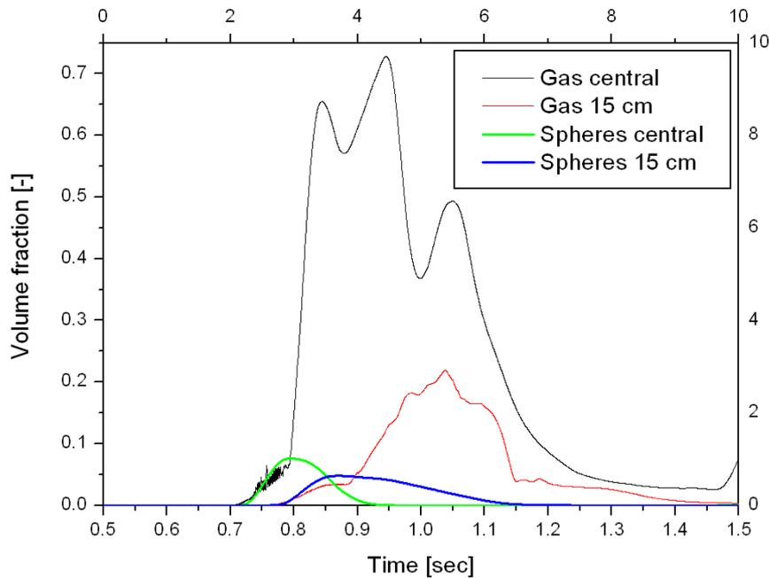
**Figure 9:** Correlation of gas and sphere volume fractions at the level of the void measurements (0.400 m).
