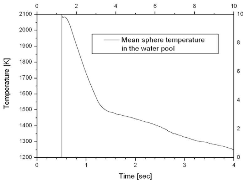
**Figure 13:** Mean sphere temperature in the water pool.
