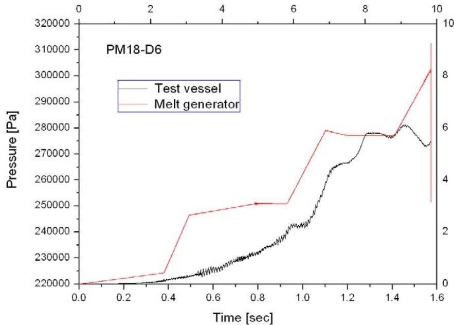
**Figure 20:** Gas pressure in the test vessel, calculated with the standard jet break-up model. The calculation is valid until blow-through occurs at 1.54 sec. The pressure in the melt generator is prescribed until 1.572 sec, i.e. except for the extremely fast changes in the end ( $>1.573$  sec). The experimental results are shown in Figure 18. Mind the difference (shift) in time scales. At about 1.2 and 1.4 sec the calculation is close to the experiment.
