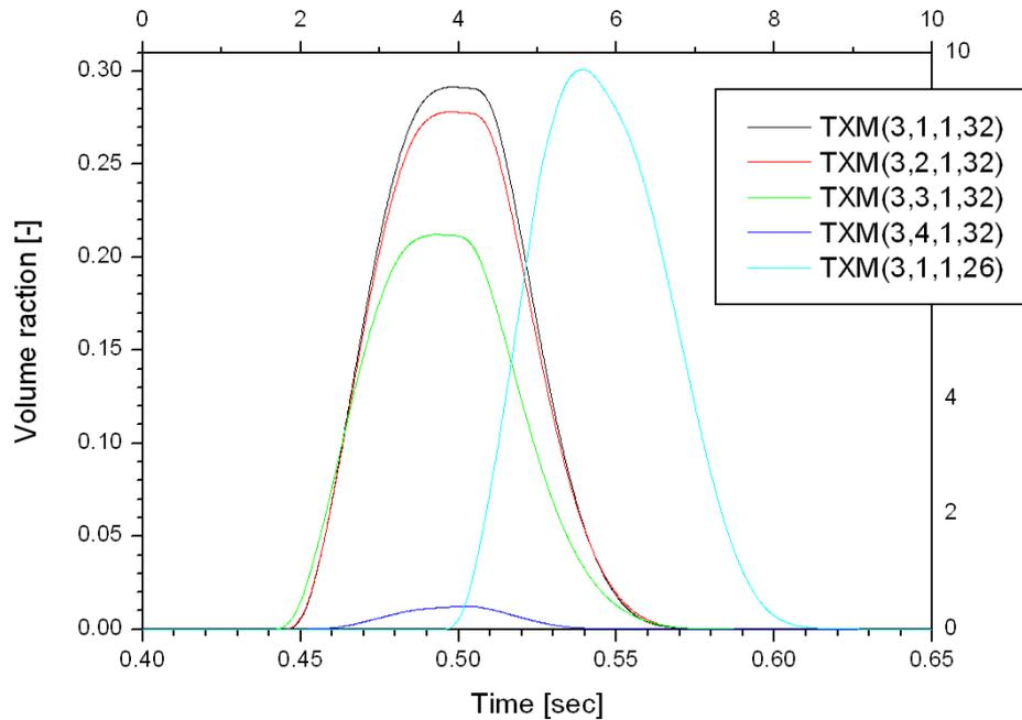
Figure 10: Volume fraction of the spheres ( $l=3$ ) in cells at two axial levels ( $k=32$ , i.e. the level of the pyrometers and  $k=26$ , i.e. the first cell above the water surface). At the upper position, the four innermost cells are shown ( $i=1, \dots, 4$ ). The legend is  $\text{TXM}(l,i,j,k)$ . The azimuthal coordinate ( $j$ ) is always 1 because cylindrical geometry has been used.
