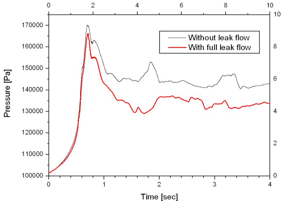
**Figure 15:** Comparison of pressure histories obtained with fully open and fully closed leak (pressure release valve).
