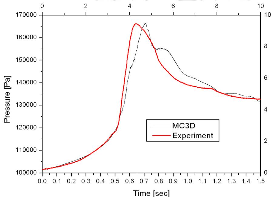
**Figure 5:** Comparison of experimental and calculated pressure development in the gas space of the test vessel in the initial phase.
