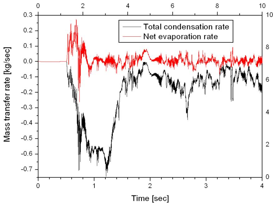
**Figure 12:** Mass transfer rates, integrated over the whole calculation domain.
