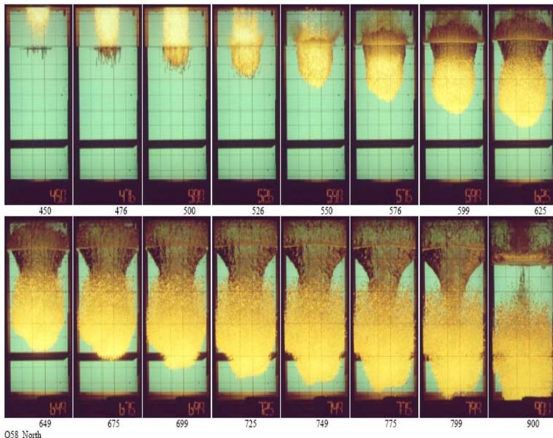
Figure 2: High-speed movie pictures of QUEOS experiment Q58. The numbers indicate the time in milliseconds.
