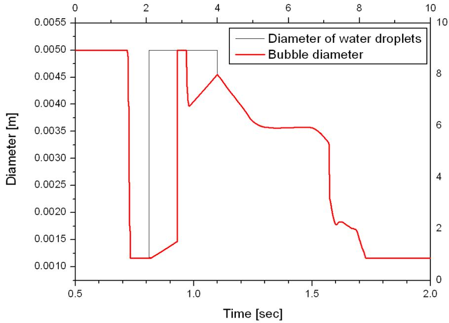
**Figure 17:** Diameters of water drops and bubbles in the cell from which the central void is taken. Minimum bubble diameter: 1.16 mm.
