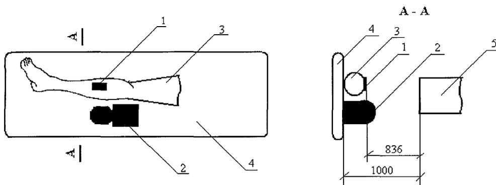
Figure 2. Calibration of the TLD detectors on the leg phantom. 1 TLD detectors, 2 VAJ-15 dosimeter, 3 Anatomic phantom, 4 Table, 5 X-ray tube. The phantom and the dosimeter were placed consecutively in the measuring point.
