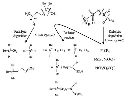
Fig. 2: Proposition of a degradation scheme of ionic liquid  $[\text{MeBu}_3\text{N}][\text{Tf}_2\text{N}]$
