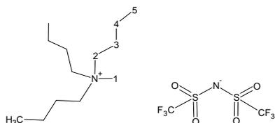
Fig. 1: Ionic liquid used: cation Methyltributylammonium  $\text{MeBu}_3\text{N}^+$  and anion bis(trifluoromethylsulfonyl)imide  $\text{Tf}_2\text{N}^-$
