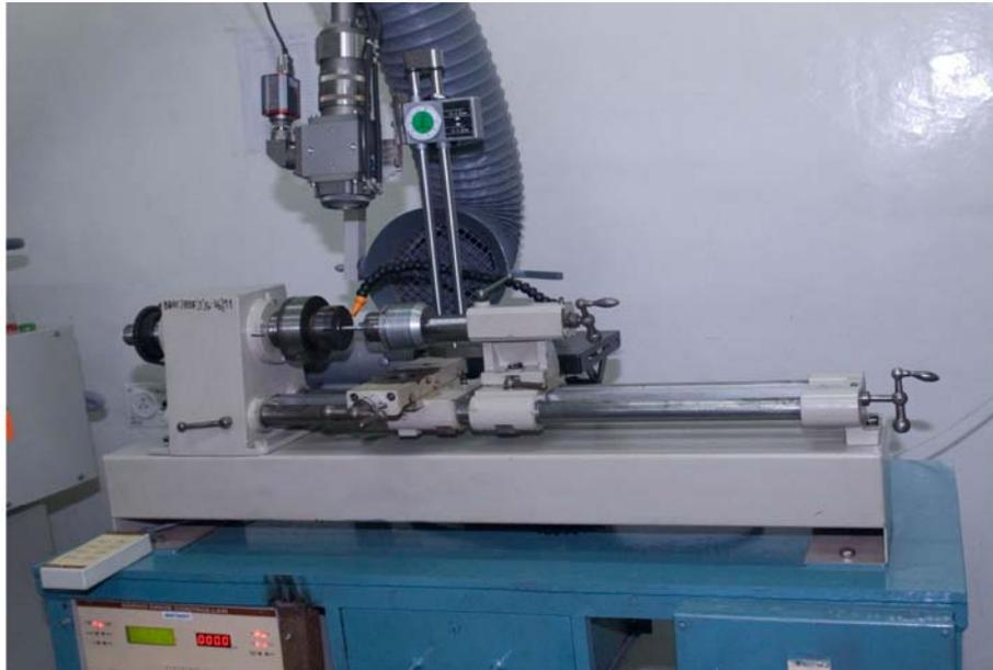
**Figure 4 Laser Weld setup showing processing optics and
