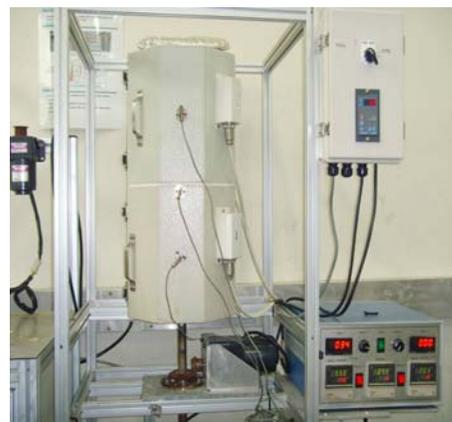
Fig.2. Testing apparatus for Cs/Sr concentration by zone freezing (vertical Bridgman) method.
