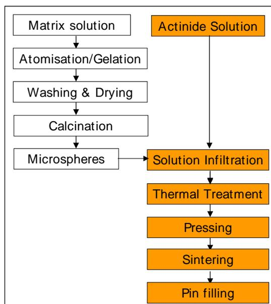
Fig. 2. Schematic flow sheet of the reference fabrication process of the MA-chain.
