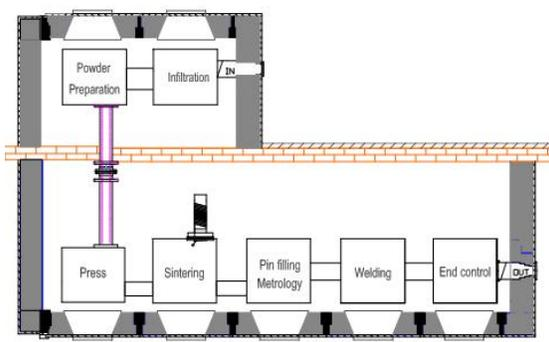
Fig. 1. General lay-out of the MA laboratory
