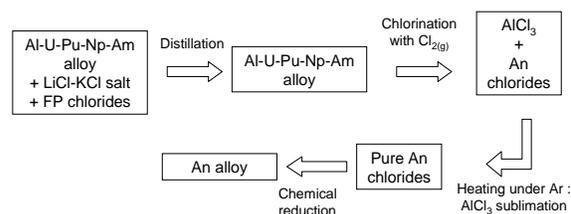
Fig. 1: Principle of the chlorination route
