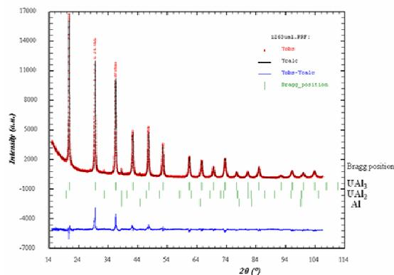
Fig. 7: X-Ray diffractogram of the U-Al alloy prepared with arc furnace and used as input material.
