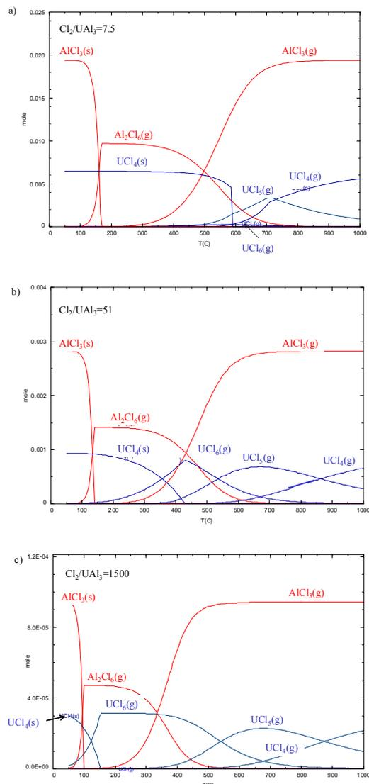
Fig. 4: Chlorination of  $\text{UAl}_3$  alloys - Calculation of the evolution of the amount of chloride compounds with temperature and  $\text{Cl}_2/\text{UAl}_3$  molar ratio. Initial conditions: 1  $\text{dm}^3$  reactor containing 2000 - 300 - 10 mg of solid  $\text{UAl}_3$  alloy and 4.843  $10^{-2}$  mol of  $\text{Cl}_2(\text{g})$  ( $P=1.2$  bars at  $25^\circ\text{C}$ ).
