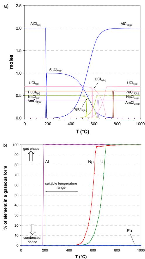
Fig. 5: Sublimation of  $\text{AlCl}_3$  from the chloride mixture. a) Evolution of the composition with T. b) Evolution of the volatilization with T. Initial conditions: mixture of 1 mole of An chlorides, 2 moles of  $\text{AlCl}_3$  and Ar (1 atm).
