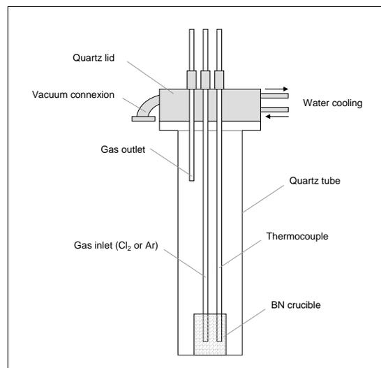
Fig. 6: Experimental set-up for chlorination – Quartz reactor
