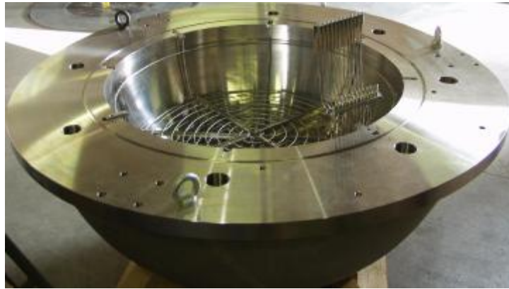
Figure 2: LIVE volumetric heating system
