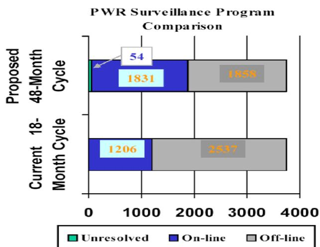
Fig.1 Possible re-categorization of maintenance items to enable 48-month maintenance cycle [3]
