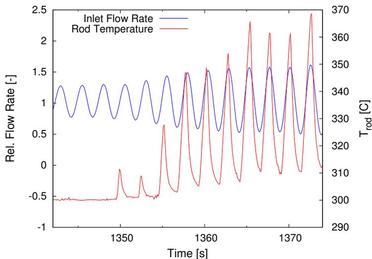
Figure 7: KATHY measured inlet flow rate and cladding temperature.
