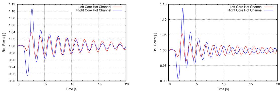
Figure 5: Power oscillations in opposite core regions after an out-of-phase perturbation for two different cases.
