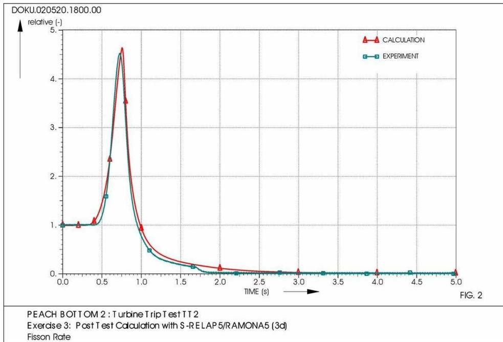
Figure 10: Measured and calculated reactor power in the Peach Bottom turbine trip benchmark
