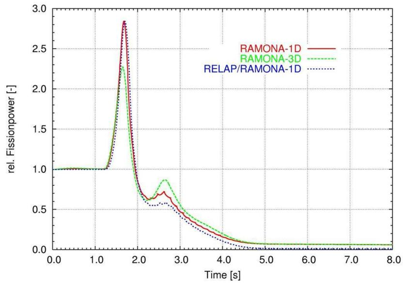
Figure 12: Comparison of the transient reactor power during the loss of the main heat sink with 1D and 3D representation of the reactor core.
