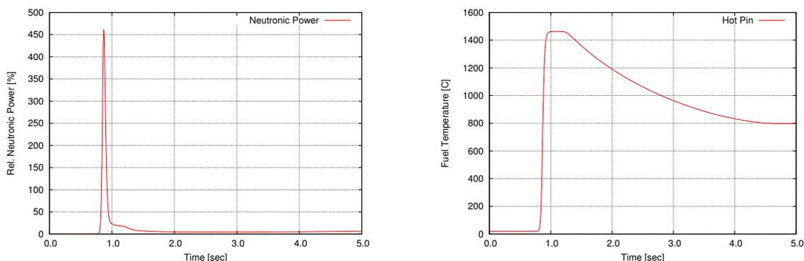
Figure 8: Transient values of neutronic power (left) and Fuel Temperature (right) during a typical RIA.
