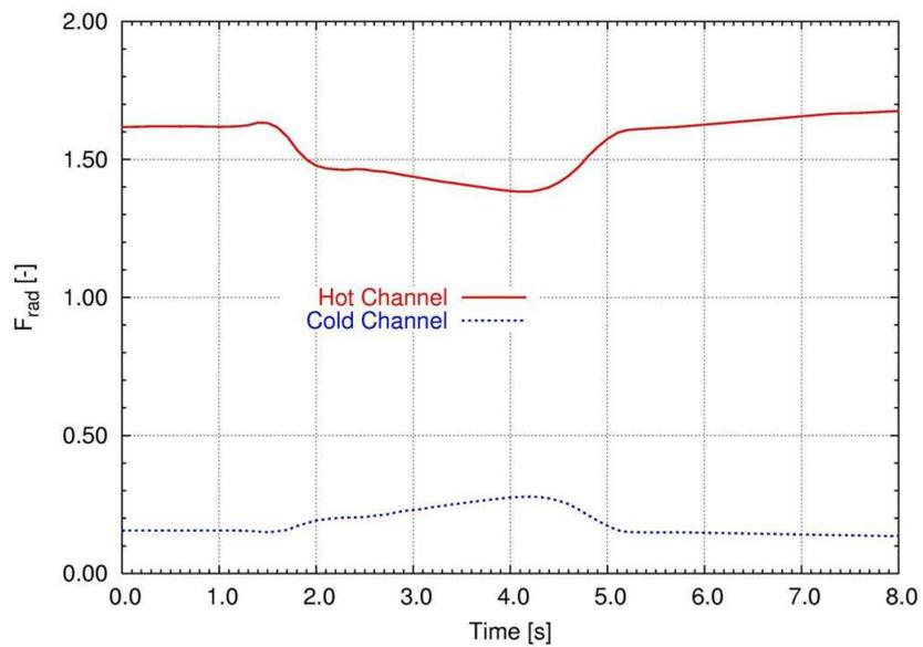
Figure 13: Transient values of the radial power factor during the loss of the main heat sink with a 3D representation of the reactor core.
