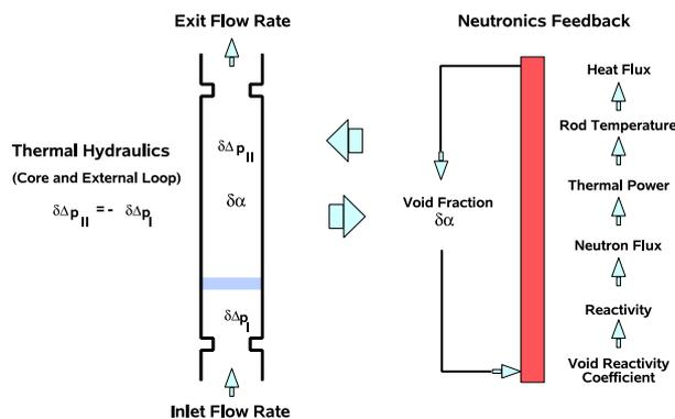
Figure 3: Feedback mechanisms of BWR stability.
