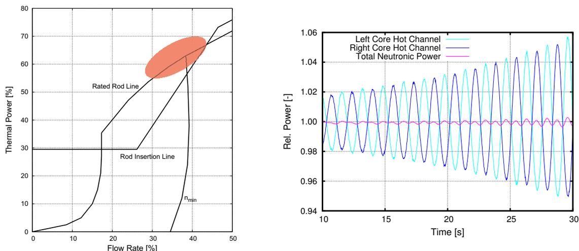
Figure 2: Left: Schematic representation of a BWR power/flow map and region (red marked) sensitive to power oscillations. Right: Power oscillations in opposite core regions and core average power signal.
