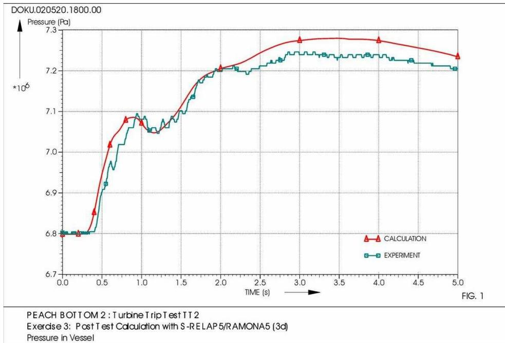
Figure 11: Measured and calculated reactor pressure in the Peach Bottom turbine trip benchmark
