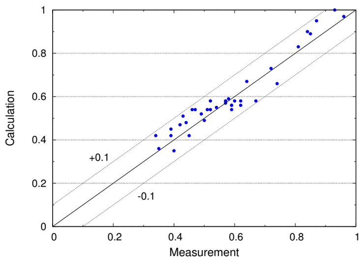
Figure 4: Comparison of decay ratios from measurements and from RAMONA analyses.
