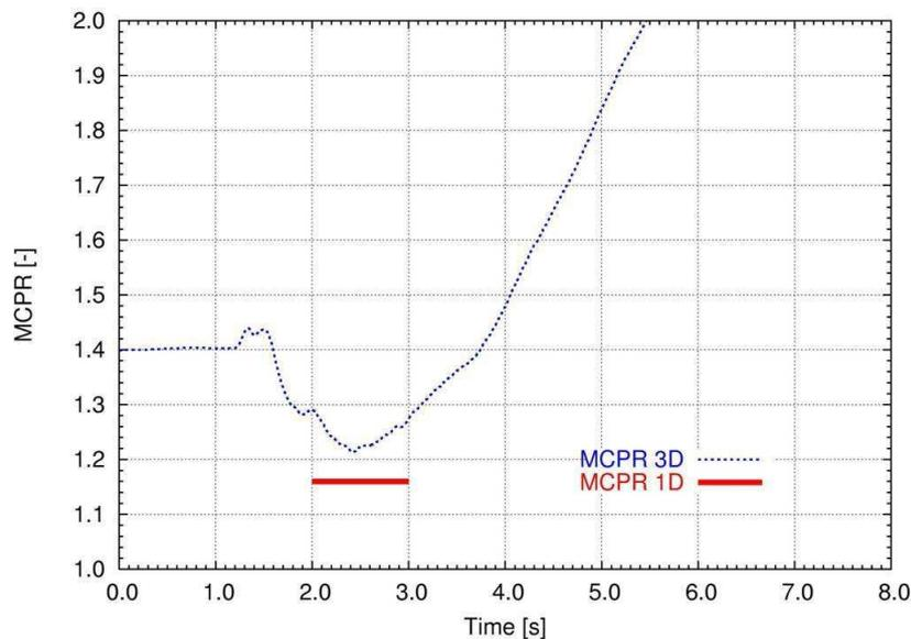
Figure 14: Transient minimal critical power ratio (MCPR) during the loss of the main heat sink with a 3D representation of the reactor core in comparison with the value out of 1D calculations.
