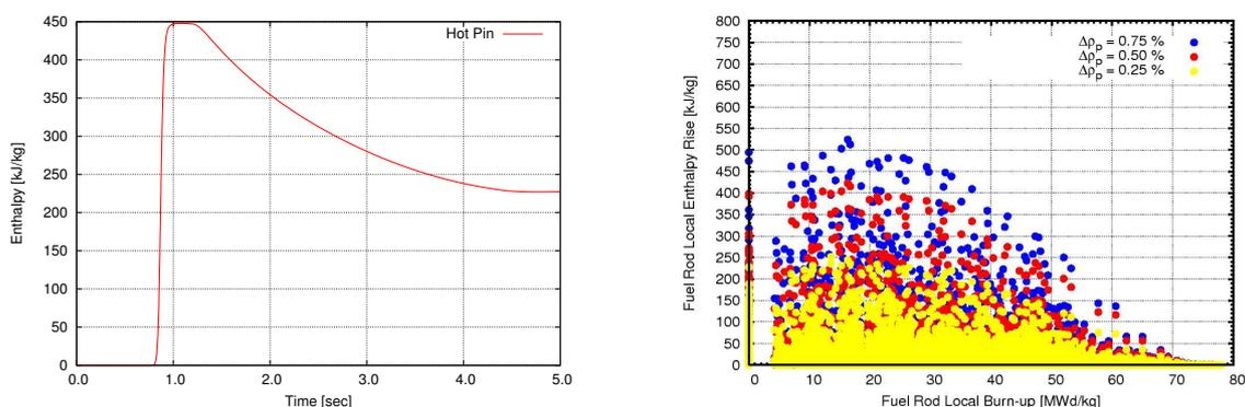
Figure 9: Left: Transient values of enthalpy during a typical RIA. Right: Fuel rod local enthalpy increase vs. fuel rod local burn-up for different prompt reactivity insertions.
