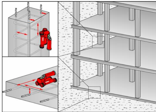
Figure 6: Checking cover and rebar layout
