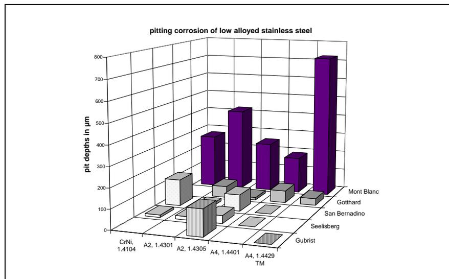
Figure 1: Pitting corrosion after two years of exposure
