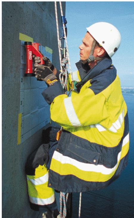
Figure 5: Location detection of rebar
