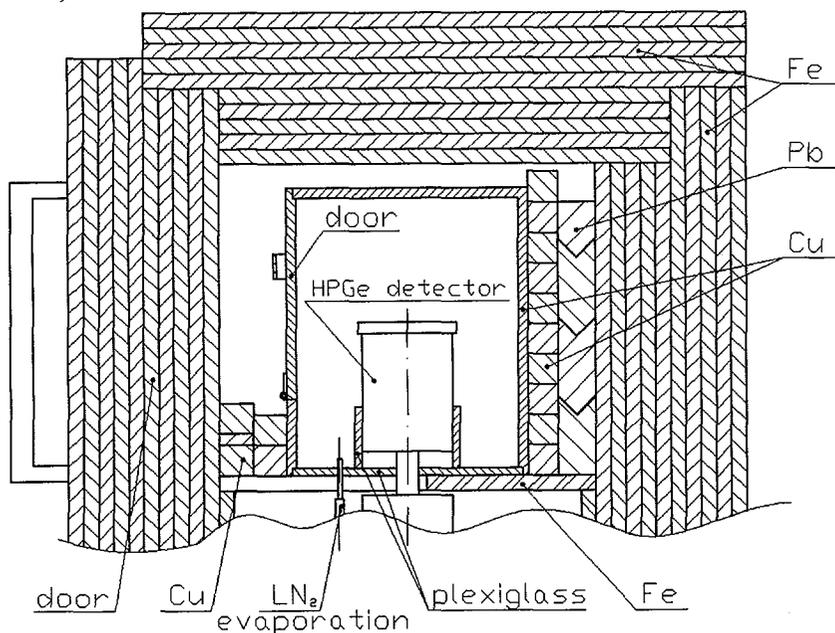
Figure 1. Schematic representation of the adjusted additional shielding – Side view
