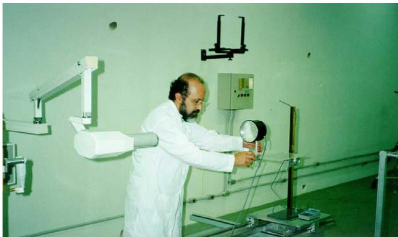
**Figure 4** – Set-up for calibration of radiodiagnostic ionization chambers in IEC reference radiations at the LCD/CDTN (a: lead housing x-ray tube; b: transmission chamber; c: lead collimator; d: reference ionization chamber; e: chamber under calibration)
