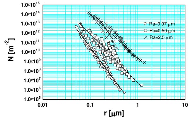
**Figure 7.** Active cavity density variation with “ $r$ ”. Refrigerant R-134a; copper tubes; all reduced pressures.
