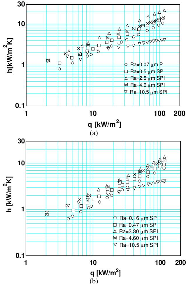
**Figure 3.** Effect of the surface roughness on a  $h$  vs  $q$  plot for refrigerants boiling on copper tubes. (a) Refrigerant R-134a;  $p_r=0.177$ ; (b) R-123;  $p_r=0.092$ .
