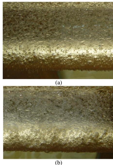
**Figure 1.** Nucleate boiling of refrigerant R-134a on a brass tube. (a)  $20\ \text{kW/m}^2$ ; (b)  $40\ \text{kW/m}^2$ .
