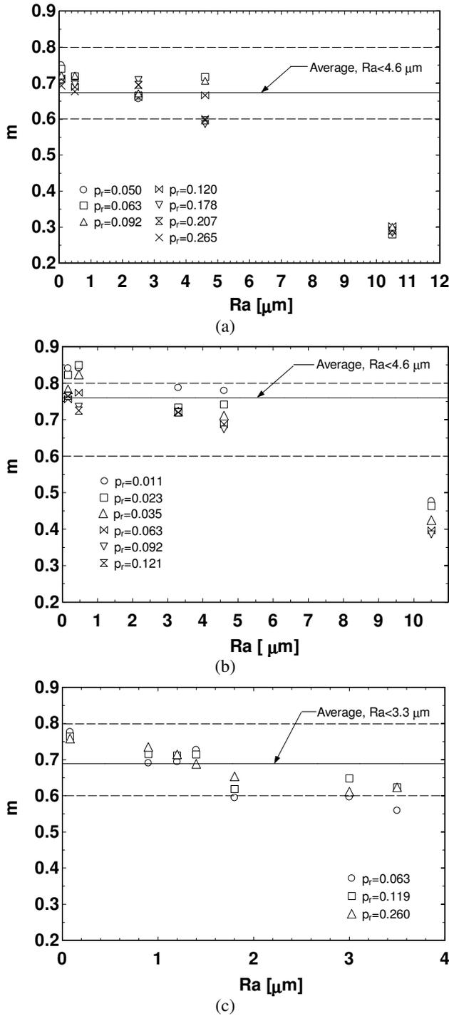
**Figure 4.** Variation of the slope of the  $h$  vs  $q$  curve, “ $m$ ”, with the average surface roughness,  $Ra$ . (a) R-134a-copper; (b) R-123-copper; (c) R-134a-brass.
