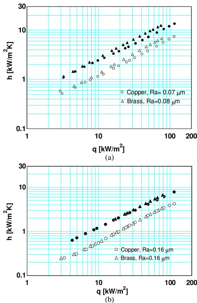
**Figure 2.**  $h$  vs  $q$  curves for boiling on copper and brass tubes. (a) Refrigerant R-134a, polished surfaces,  $p_r=0.063$  and  $0.260$ ,  $Ra=0.07\ \mu\text{m}$  and  $0.08\ \mu\text{m}$ ; Refrigerant R-123, scaled surfaces,  $p_r=0.011$  and  $0.092$ ,  $Ra=0.16\ \mu\text{m}$ . Symbols: Blank: lower pressure; blackened: higher pressure.
