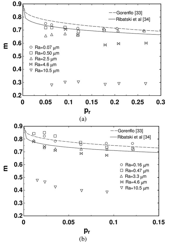
**Figure 5.** Data of Figs. 4 (a) and (b) plotted in terms of the reduced pressure. (a) R-134a-copper; (b) R-123-copper.
