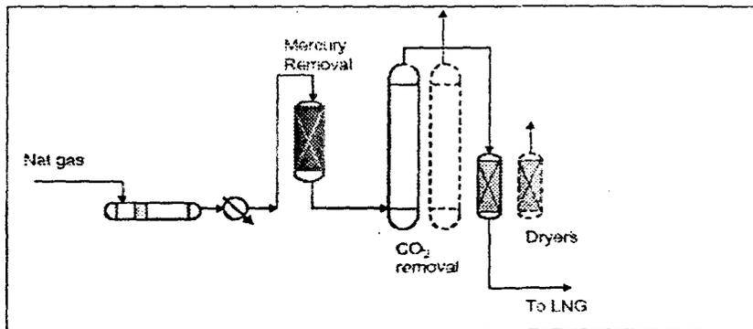
Figure (19): Location of Mercury Removal before Acid Gas Removal Unit
