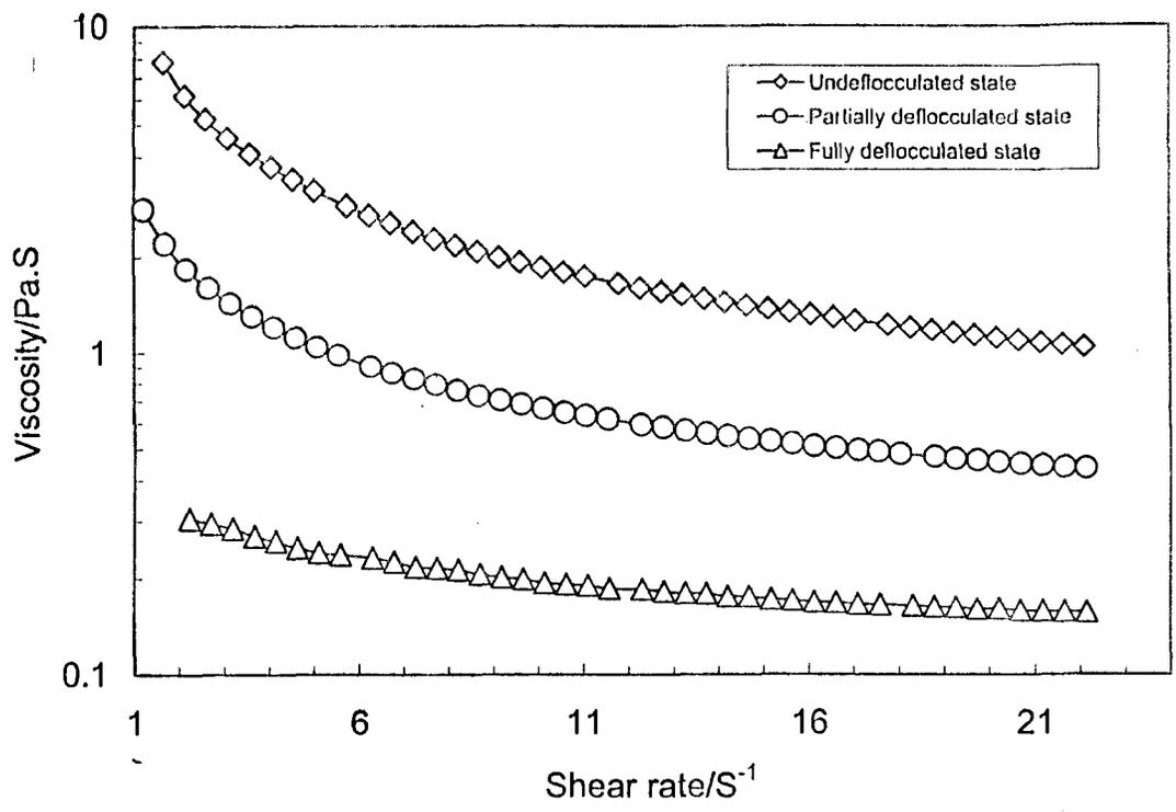
Fig. (5) Viscosity of alumina suspension with different states as a function of shear rate at PH value of 9.4
