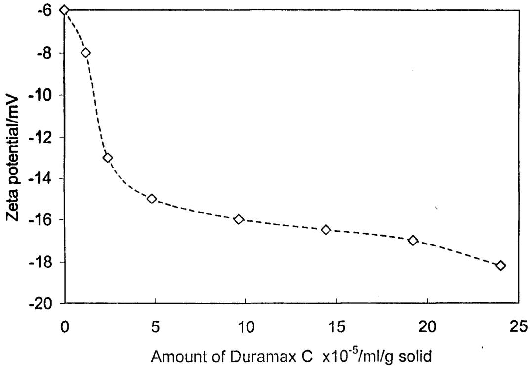
**Fig.(2) Variation of zeta potential of alumina suspension as a function of Duramax C concentration at pH value of 9.4**
