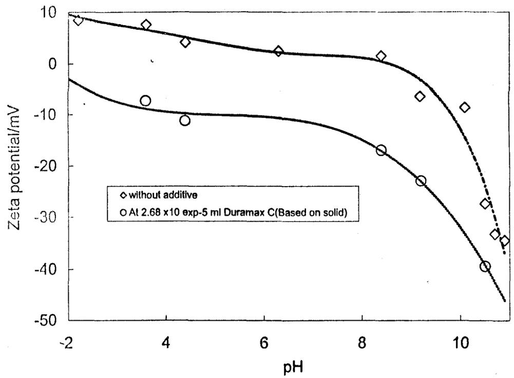
Fig. (1) Variation of zeta potential of alumina suspension as a function of pH
