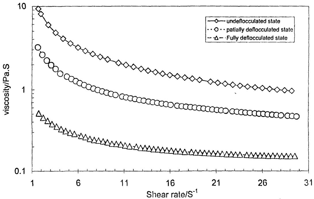
Fig. (4) Viscosity of alumina suspension with different states as a function of shear rate at PH value of 8.4
