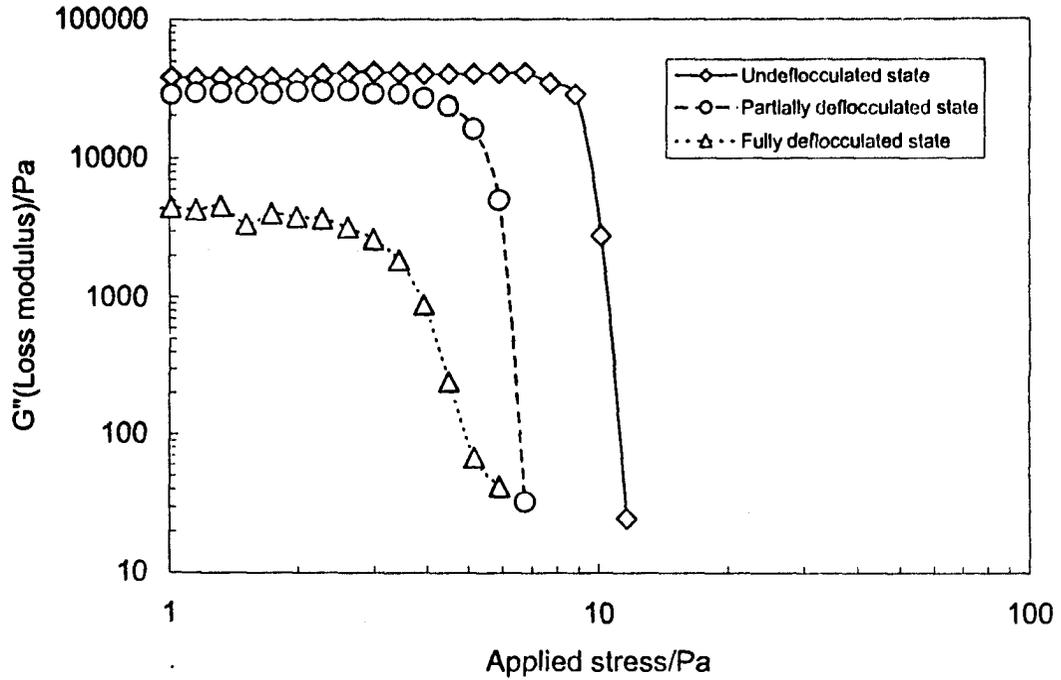
Fig.(7) Dynamic stress sweep in term of viscous modulus for alumina suspension with different states as a function of applied stress at pH value of 9.4
