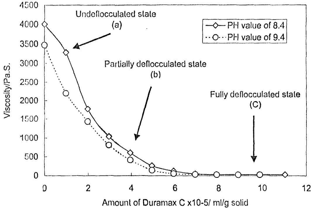
Fig. (3) Viscosity of alumina suspension as a function of Duramax concentration at pH value of 8.4 and 9.4
