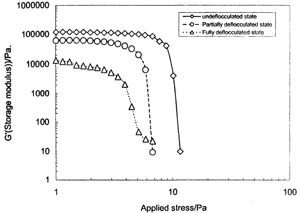
Fig.(6) Dynamic stress sweep in term of elastic modulus for alumina suspension with different states as a function of applied stress at pH value of 9.4
