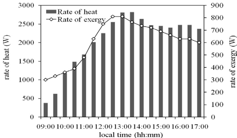
Figure 5: The rates of heat and thermal exergy stored in the heat storage unit during the charging period
