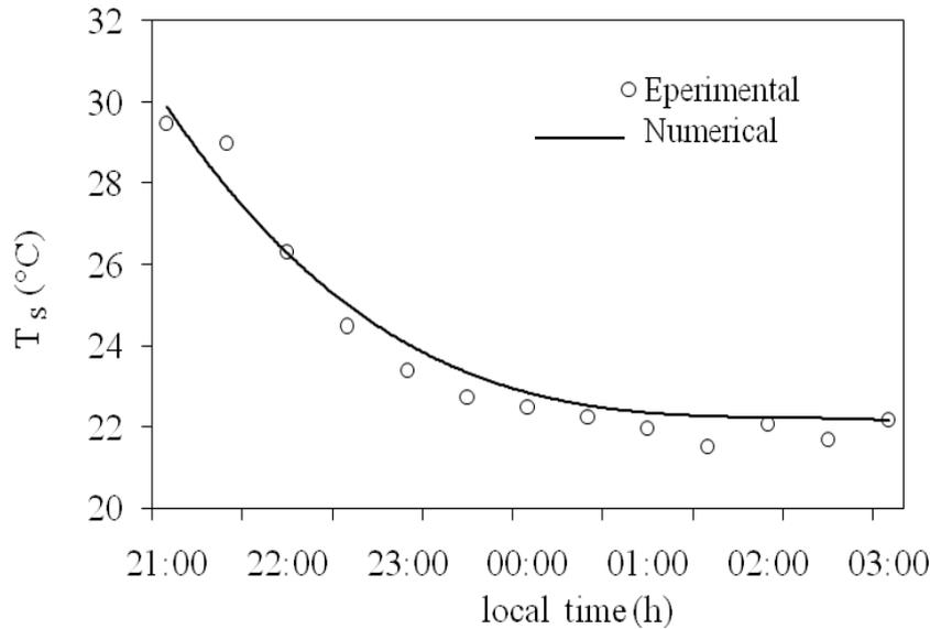
Figure 7: Evolution of the sand temperature at 40 cm-depth during the discharging phase
