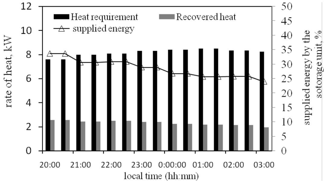
Figure 9: The changes of the total heat requirement of the tunnel greenhouse and the rate of heat recovered from the heat storage unit during the discharging period
