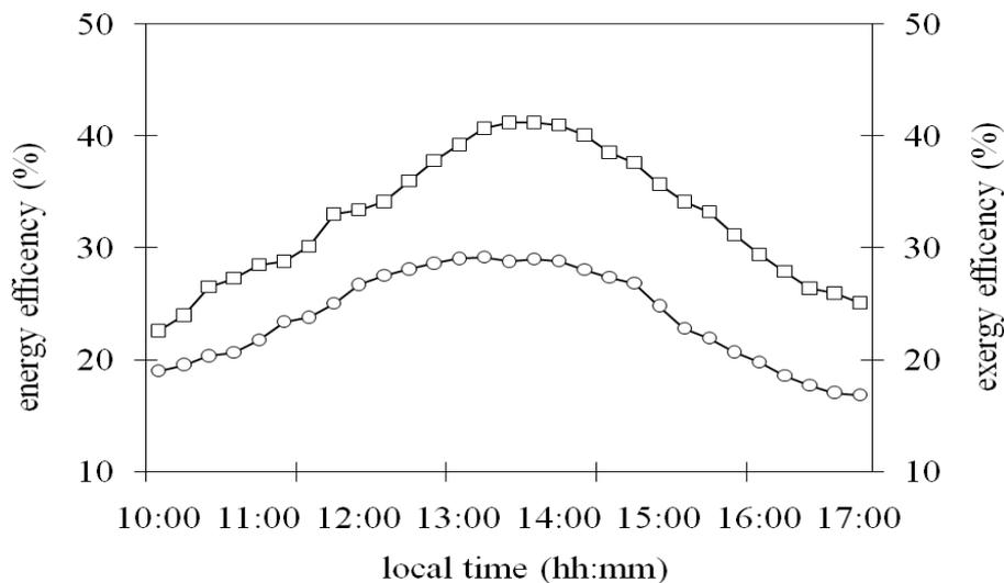
Figure 6: The change of the net energy and exergy efficiencies for the charging period:  $\square$ , energy efficiency,  $\circ$  exergy efficiency
