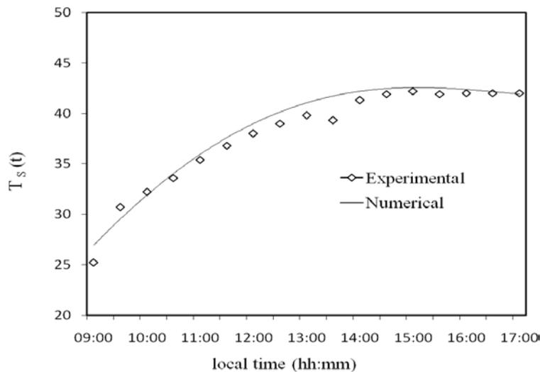
Figure 4: Evolution of the sand temperature at 50 cm-depth during the charging phase
