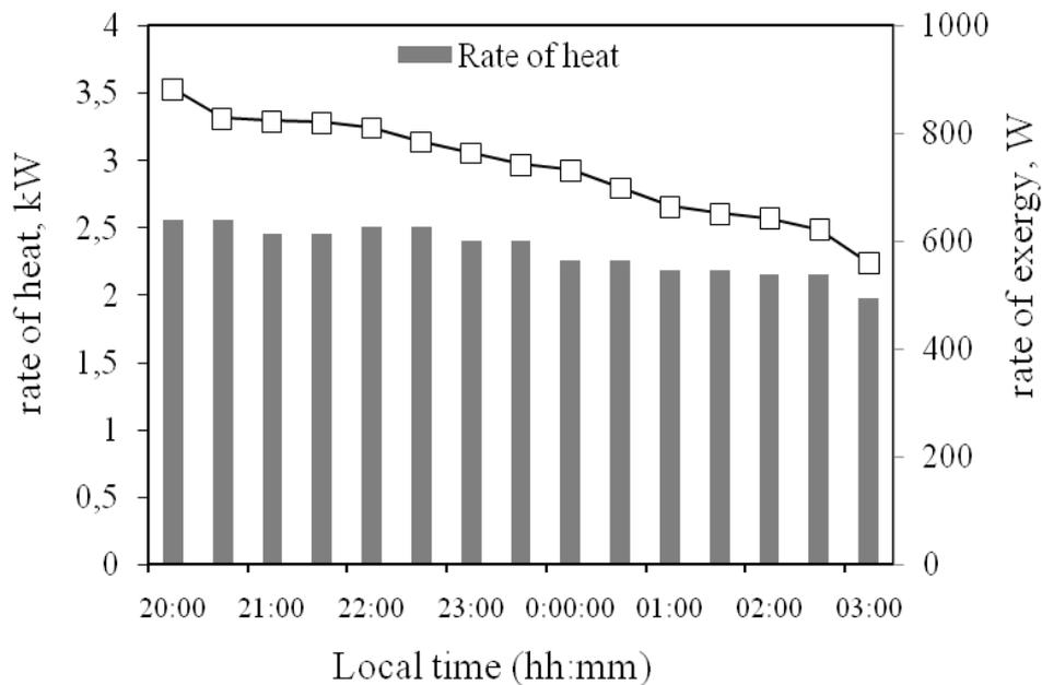
Figure 8: The rates of heat and thermal exergy recovered from the heat storage unit for the discharging period
