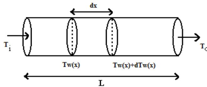
Figure 1. Diagram of an element of a heat exchanger
