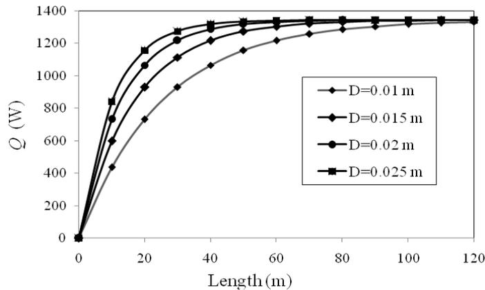
Figure 4. Heat extracted from ground according to exchanger length and diameter
