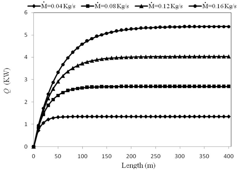
Figure 2. Heat extracted from ground according to the exchanger length and flow rate
