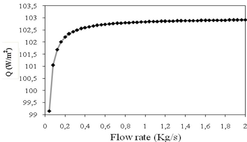
Figure 3. Heat extracted from ground according to the exchanger length and flow rate
