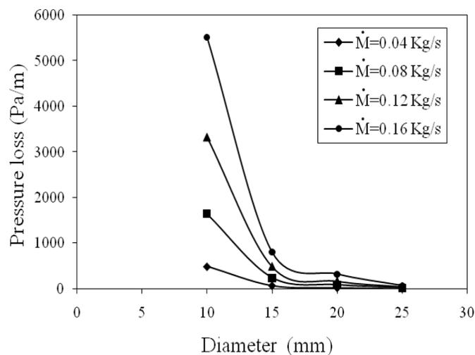
Figure 3. Pressure loss according to the flow rate and Diameter
