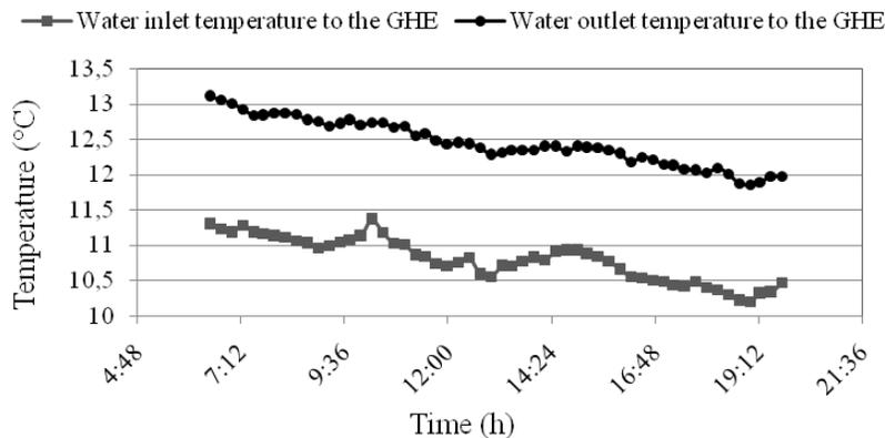
Figure 5. Comparison between water inlet and outlet temperatures of the GHE
