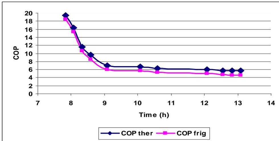
Figure 7. Evolution of the refrigerating and thermal COP vs the hour
