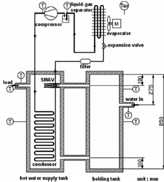
Figure 1. Schematic diagram of the FRHP. (Huang 2008)
