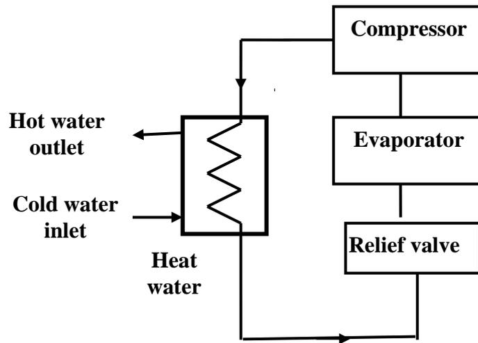
Figure 4. Diagram of the modified refrigerating circuit to heat water
