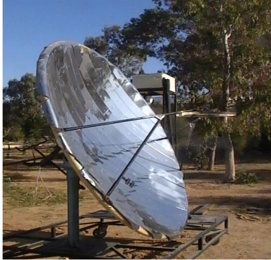
Fig. 1. Photograph of the experimental solar cooker
