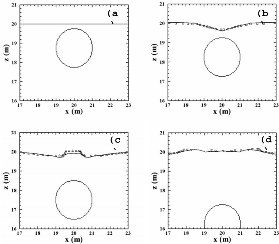
Figure 3. Water sinking of a horizontal cylinder. The simulated free surface profiles in the vicinity of the cylinder (— solid line) compared to Lin (2007) numerical results (symbols); a)  $t = 0.00$  s; b)  $t = 1.28$  s; c)  $t = 3.20$  s; d)  $t = 6.41$  s.
