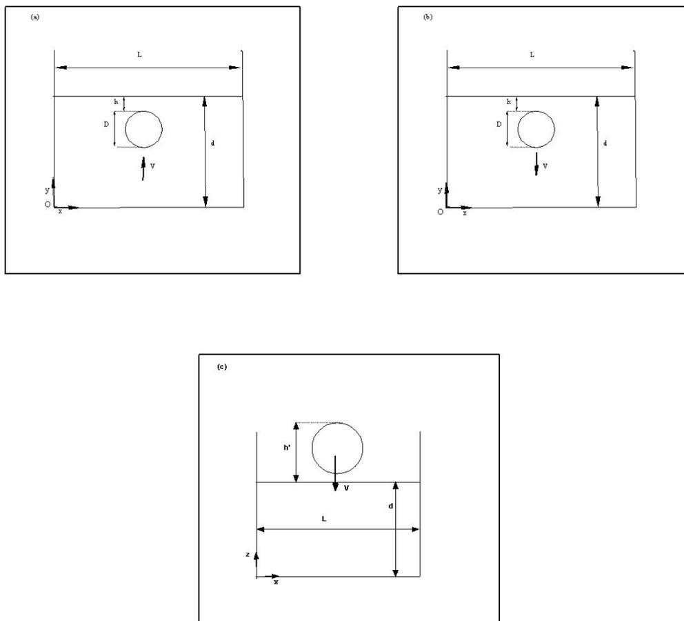
Figure 1. Definition sketch of the moving horizontal cylinder
