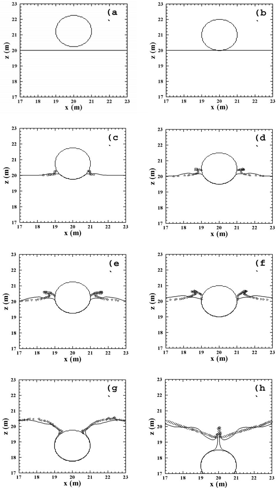
Figure 4. Water impact and entry of horizontal cylinder. The simulated free surface profiles in the vicinity of the cylinder (— solid line) compared to Lin (2007) numerical results (symbols); a)  $t = 0.00$  s; b)  $t = 0.25$  s; c)  $t = 0.50$  s; d)  $t = 0.75$  s; e)  $t = 1.00$  s; f)  $t = 1.25$  s; g)  $t = 2.50$  s; h)  $t = 3.75$  s.
