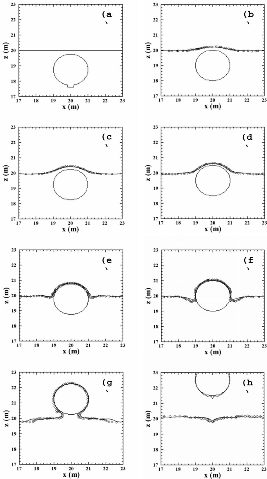
Figure 2. Water exit of horizontal cylinder. The simulated free surface profiles in the vicinity of the cylinder (— solid line) compared to Lin (2007) numerical results (symbols); a)  $t = 0.00$  s; b)  $t = 0.64$  s; c)  $t = 1.28$  s; d)  $t = 1.92$  s; e)  $t = 2.56$  s; f)  $t = 3.20$  s; g)  $t = 6.41$  s; h)  $t = 9.61$  s.
