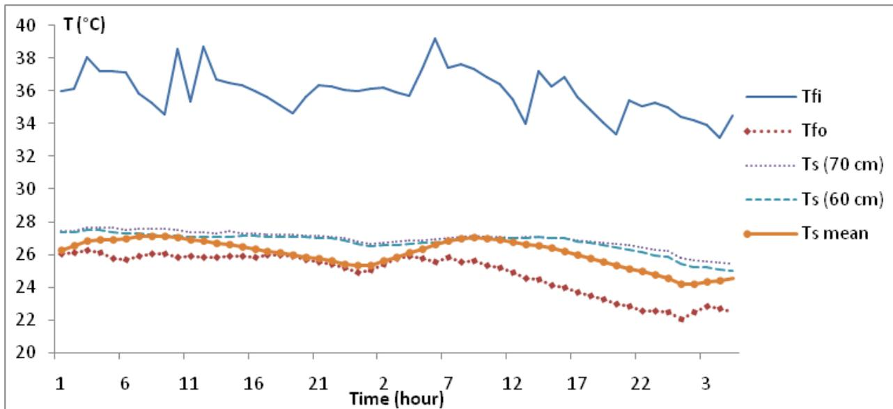
Figure 5. Variation of the soil temperature at 60 and 70 cm depths when the soil was heated at 36°C
