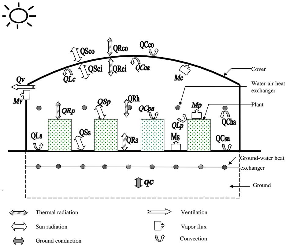
Figure 2. A schematic illustration of heat and mass fluxes existing in the greenhouse
