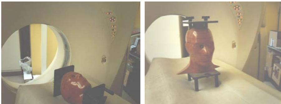
**Figure 7 : Rando head phantom used to investigate image quality.**
