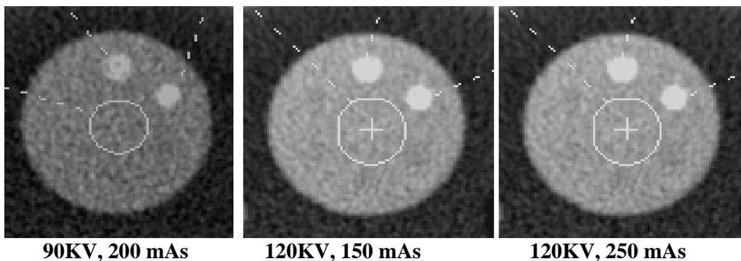
**Figure-6 : Low contrast insert images at different KV and mAs settings**
