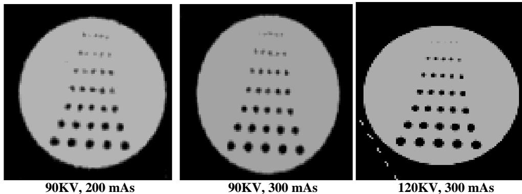
**Figure-5: Spatial resolution insert images at different KV and mAs settings**
