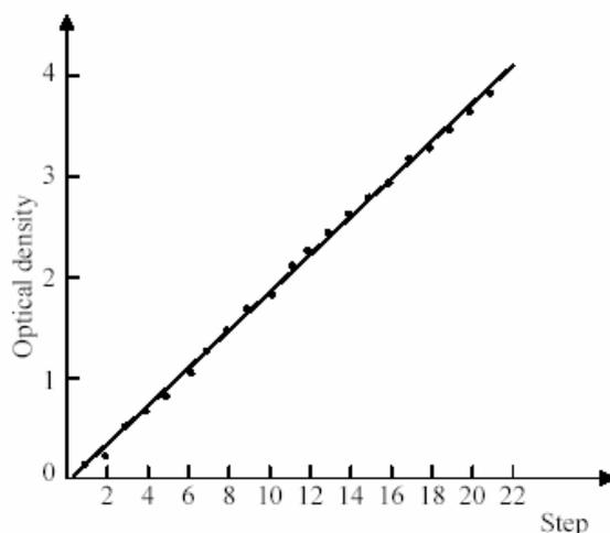
**Fig. 4 - Optical density and the 21 steps for Multidata delivered film with calibration certificate.**
