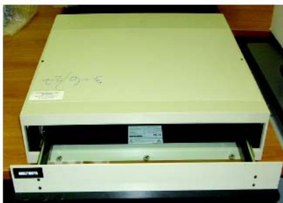
**Fig. 1 - The model 9721 Film Densitometer.**
