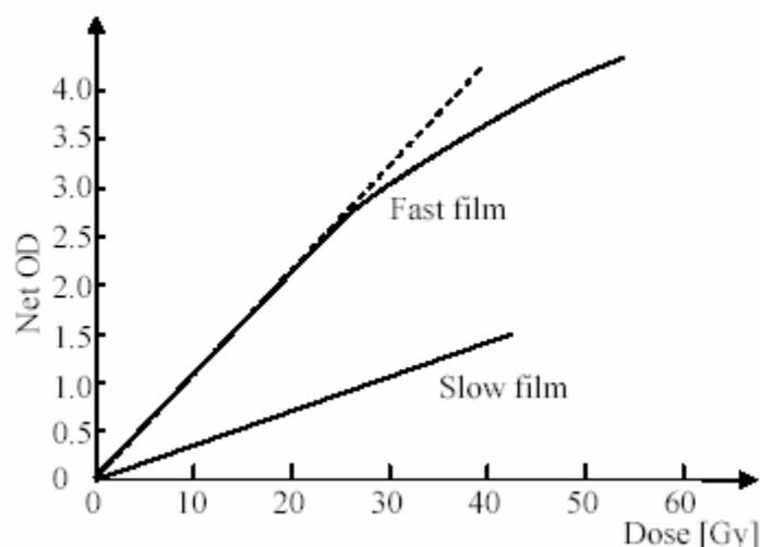
**Fig. 3 – Typical response curve, i.e. net optical density versus dose curves of radiographic films for direct x-ray exposure (Kodak 1999).**
